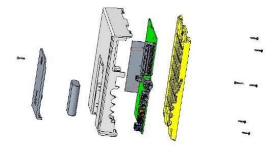
a. Align the outer contour of the bottom cover with the inner contour of the top cover, gently press the bottom cover in place, and the clips will snap the top and bottom covers together.
