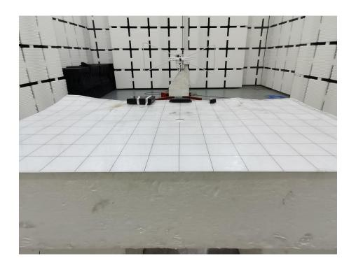
Set-up for Radiated Spurious Emission, Above 1GHz
