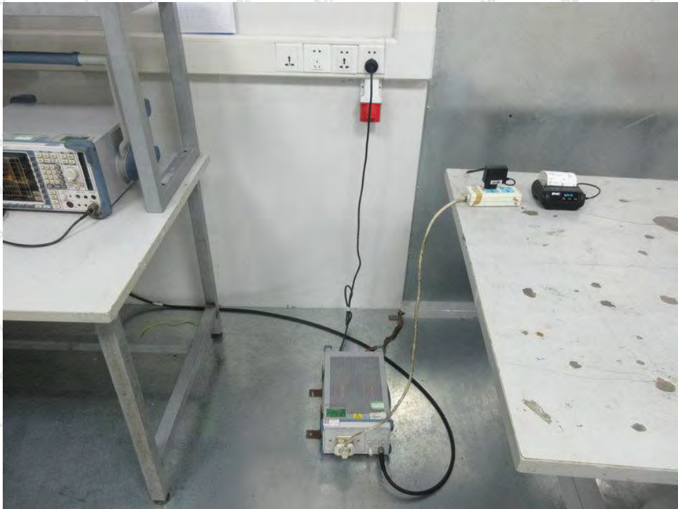
Photo of Power Line Conducted Emission Test
