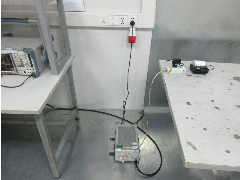
Photo of Power Line Conducted Emission Test
