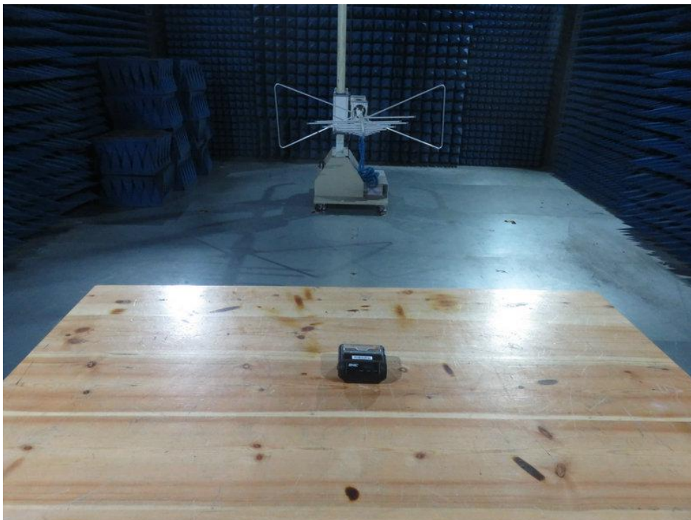
Photo of Radiation Emission Test
