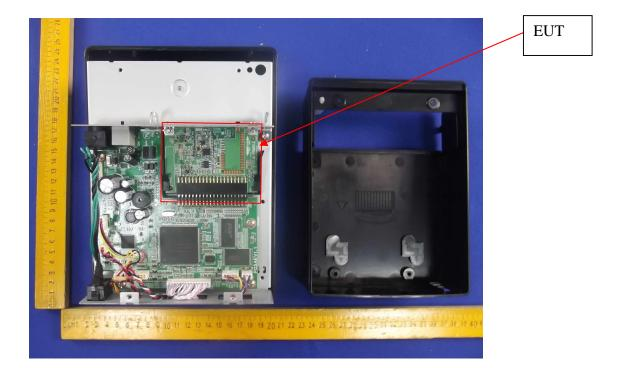
2 Photo of Radiation Emission Test
