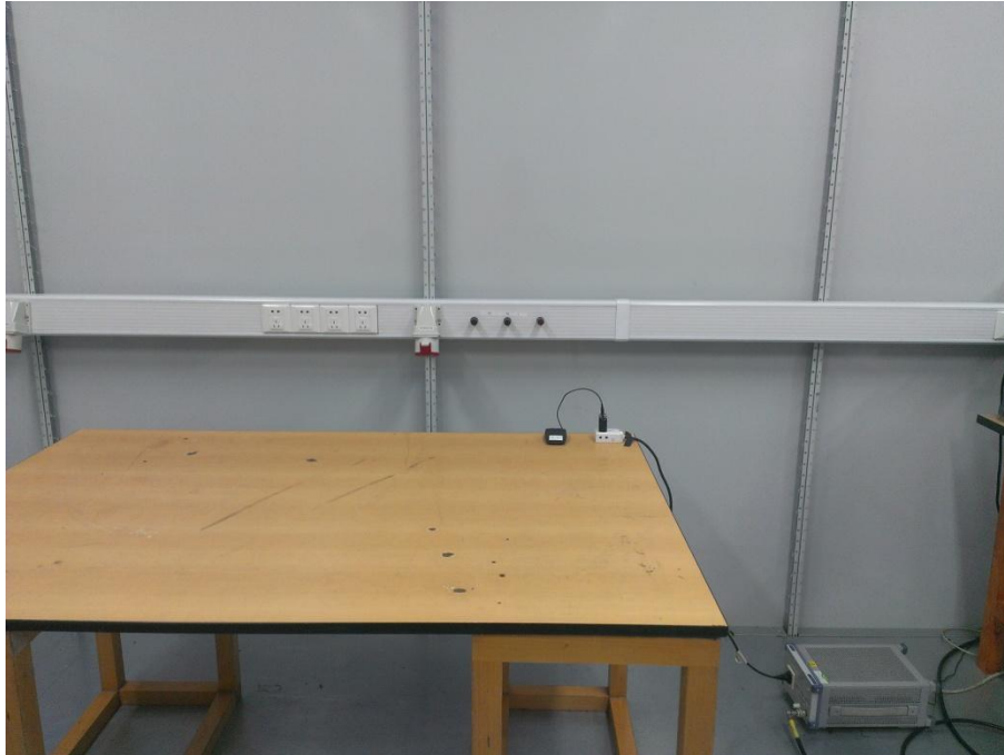
Photograph 5: Conducted Emission Test Configuration, (Below 1GHz) Back
