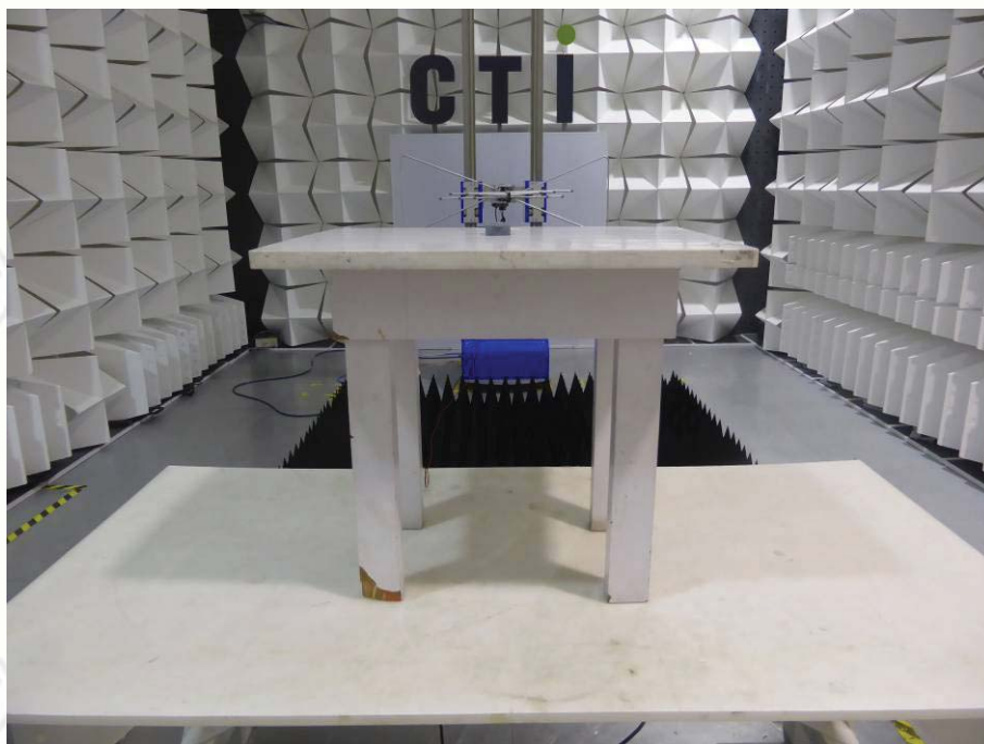
Radiated spurious emission Test Setup-1 (Below 1GHz)
