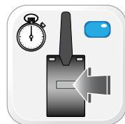
Press and release the antenna button, then press and hold the antenna button. The antenna's leds will turn solid BLUE.
