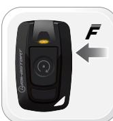
To program an additional remote as second vehicle mode: Follow steps 1 to 4. Press twice [2x] on the "F" button then press once [1x] on the LOCK button of the remote. Follow steps 6 to 9.
