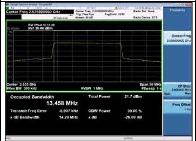
LTE band 7 - Middle CH 16QAM-15
