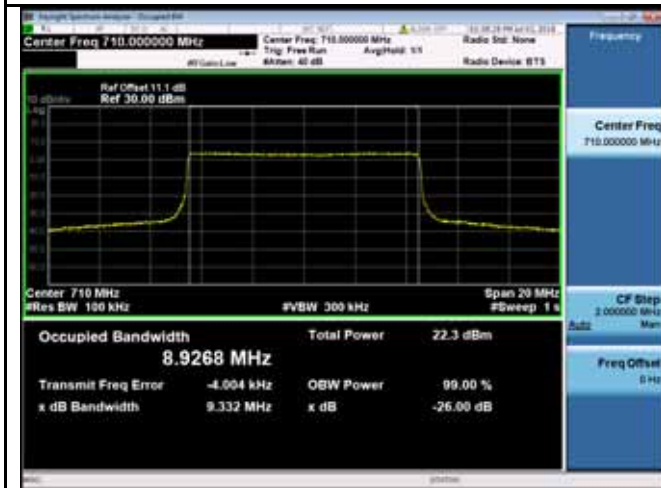
LTE band 17 - Low CH QPSK-10
