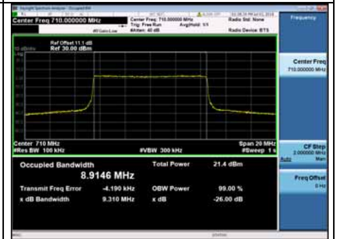
LTE band 17 - Low CH 16QAM-10
