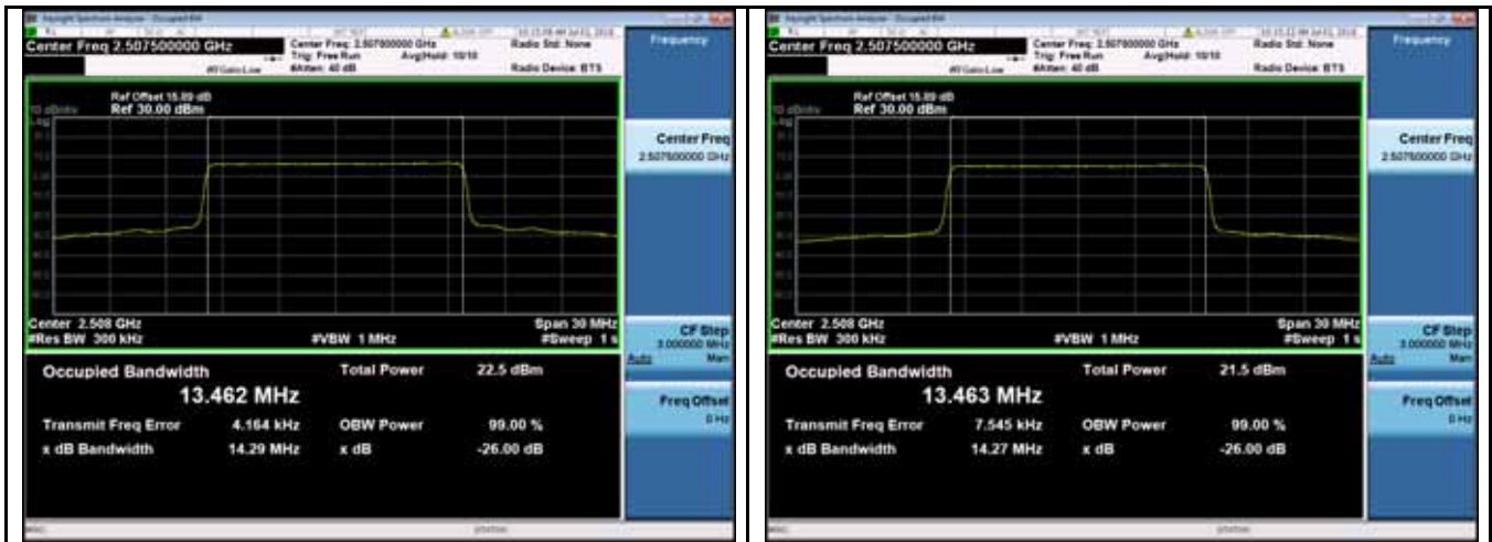
LTE band 7 - Low CH QPSK-15
