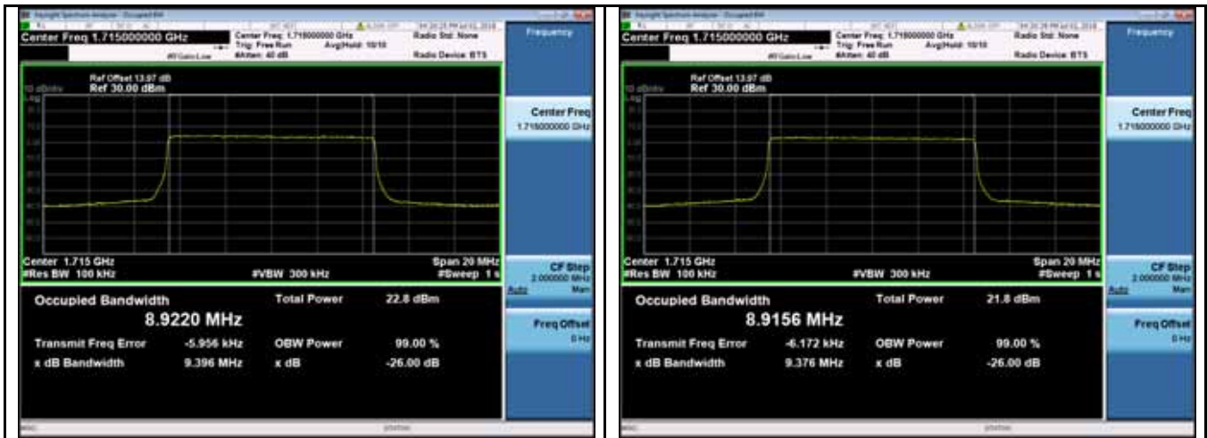
LTE band 4 - Low CH QPSK-10
