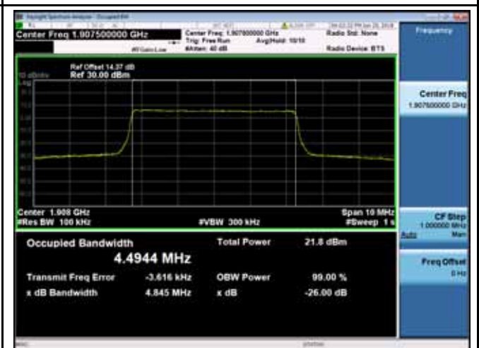
LTE band 2 - Middle CH 16QAM-5
