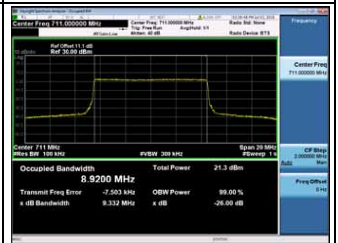
LTE band 17 - Middle CH 16QAM-10
