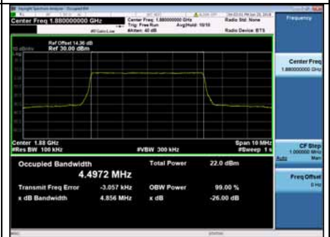
LTE band 2 - Middle CH 16QAM-5
