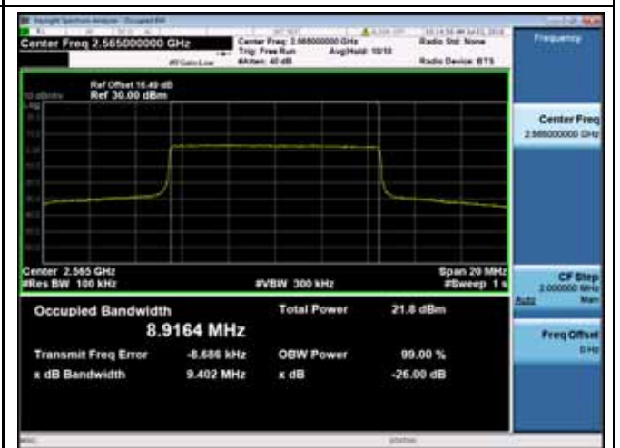
LTE band 7 - Middle CH 16QAM-10
