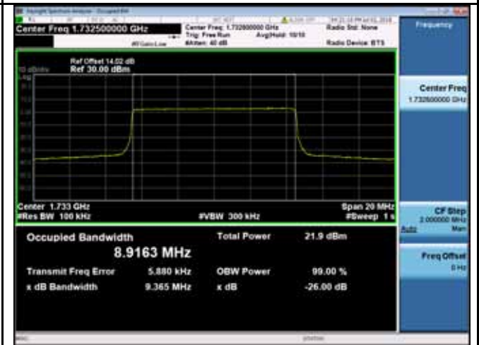
LTE band 4 - Middle CH 16QAM-10
