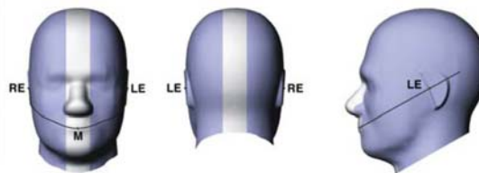
Figure 6.2 Front, back and side view of SAM
