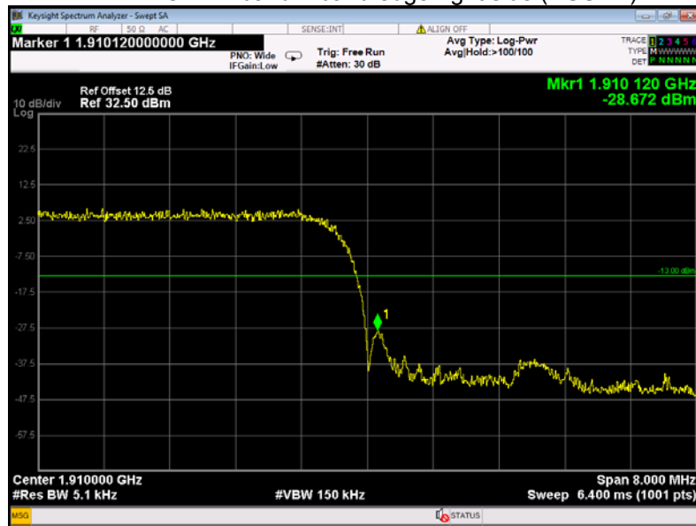
WCDMA band II band edge-right side (HSUPA)
