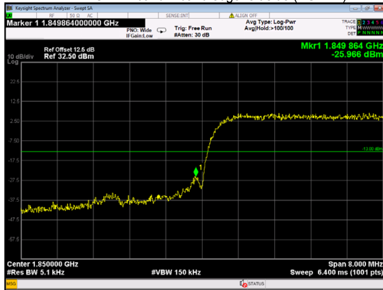
WCDMA band II band edge-left side (HSDPA)
