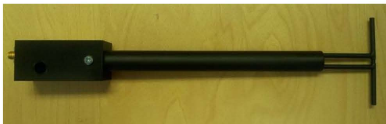
Figure 1 – MVG COMOSAR Validation Dipole
