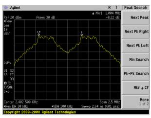
(1Mbps) Channel Separation plot on channel 00-01
