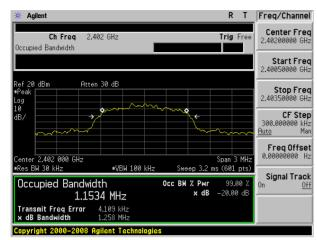
20dB Bandwidth plot on channel 39 (3Mbps)
