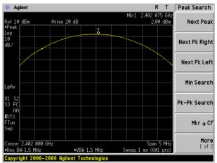
Peak output Power plot on channel 39 (2Mbps)
