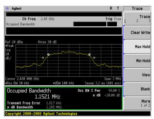
20dB Bandwidth plot on channel 78 (3Mbps)
