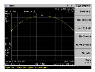
Peak output Power plot on channel 78 (1Mbps)
