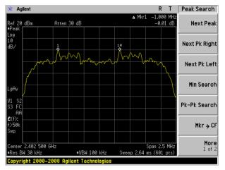
(2Mbps) Channel Separation plot on channel 39-40
