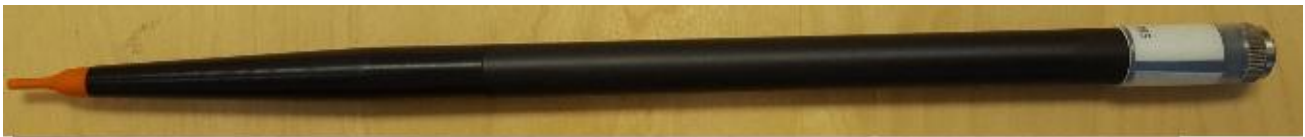
Figure 1 – MVG COMOSAR Dosimetric E field Dipole
