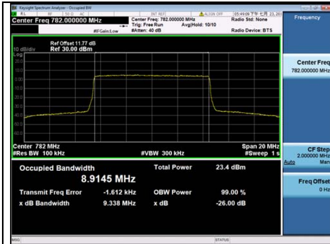
LTE band 13 - Low CH QPSK-10
