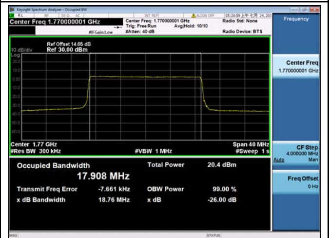
LTE band 66 - Middle CH 16QAM-20
