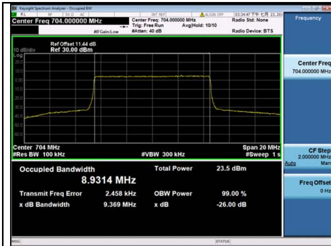
LTE band 12 - Low CH QPSK-10
