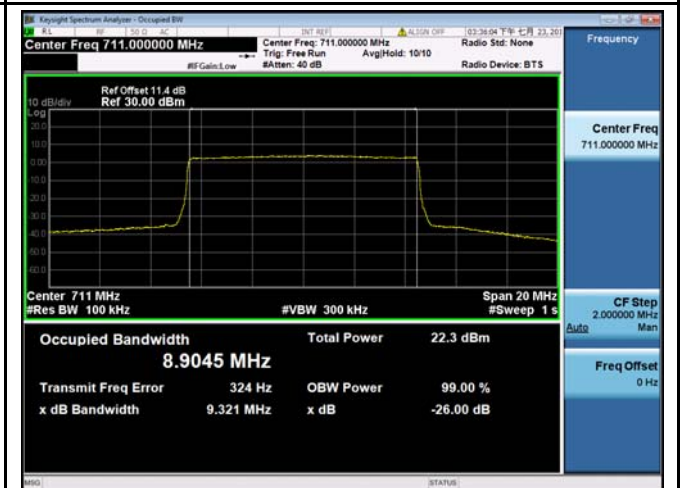
LTE band 12 - Middle CH 16QAM-10
