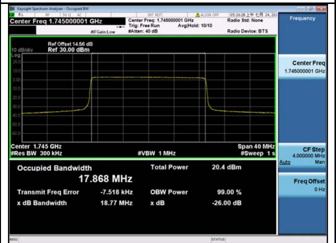
LTE band 66 - Low CH 16QAM-20
