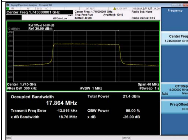
LTE band 66 - Low CH QPSK-20
