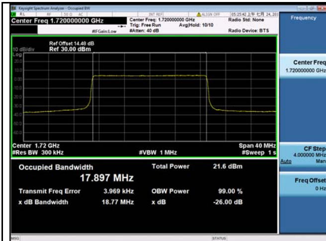
LTE band 66 - Low CH QPSK-20
