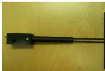
Figure 1 – MVG COMOSAR Validation Dipole
