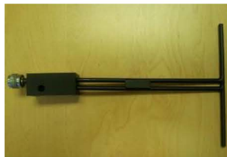
Figure 1 – MVG COMOSAR Validation Dipole
