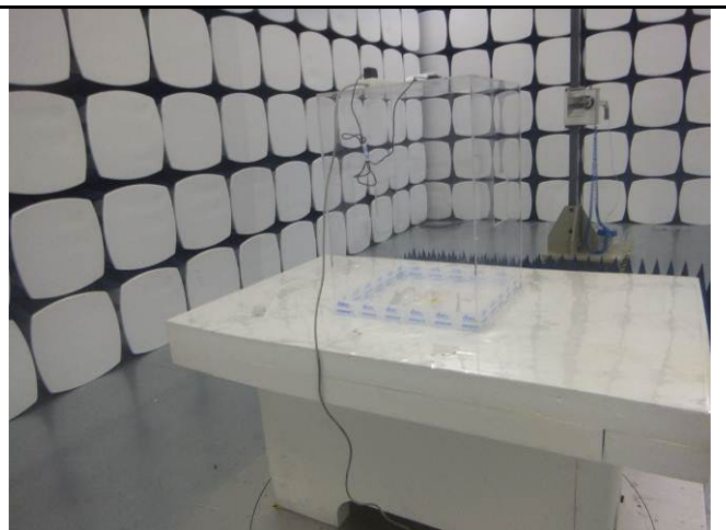
Radiated Spurious Emissions Test Setup Above 1GHz
