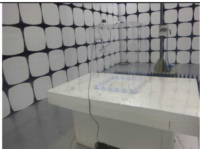
Radiated Spurious Emissions Test Setup Above 1GHz
