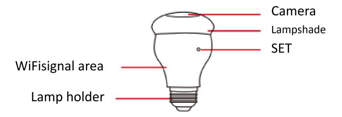
Tips one: Screw the bulb into the lamp and ensure power. Turn on and off the bulb at intervals of 1-3 seconds. After 5 cycles, it will restore into default factory setting.
