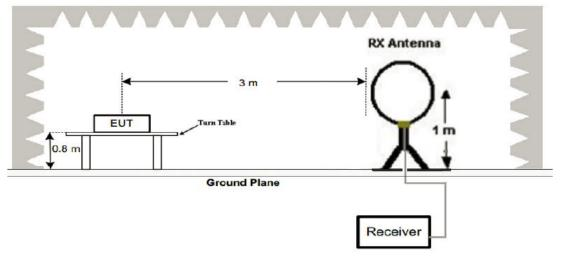
(2) Radiated Emission Test-Up Frequency 30MHz~1GHz
