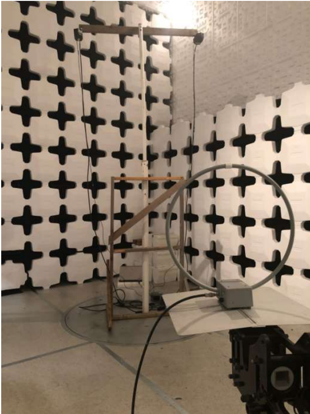
Figure 4. Radiated Emissions Below 30 MHz, 3.7 Meters
