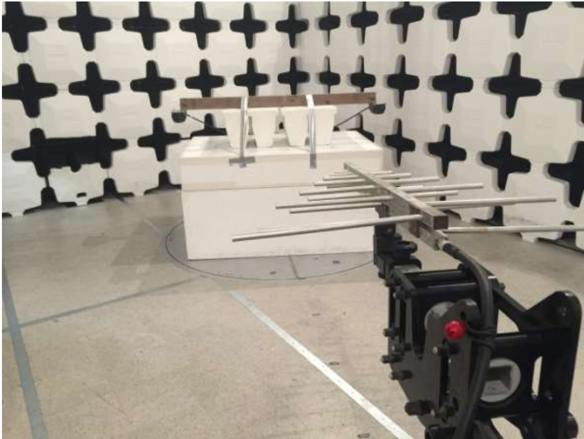
Figure 7. Radiated Emissions, 200-1000 MHz, 1 Meter
