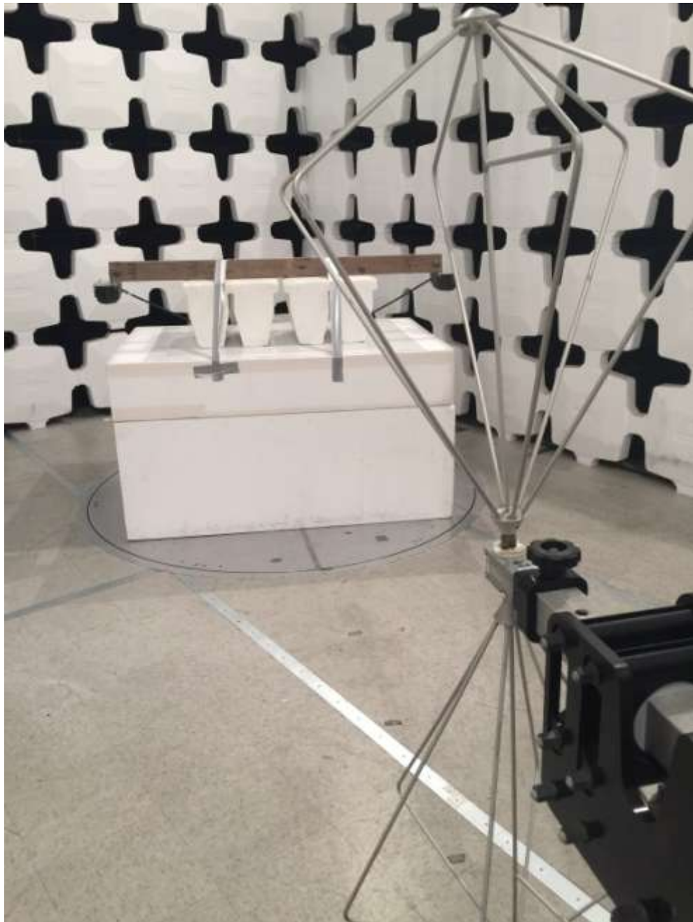
Figure 5. Radiated Emissions, 30-200 MHz, 1 Meter
