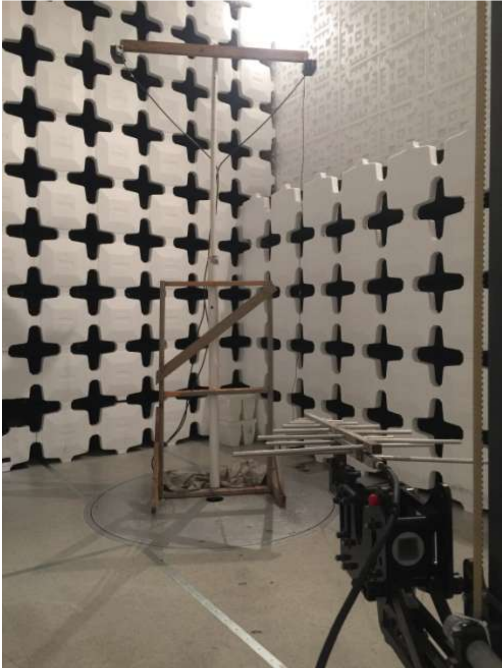
Figure 8. Radiated Emissions, 200-1000 MHz, 3.7 Meters
