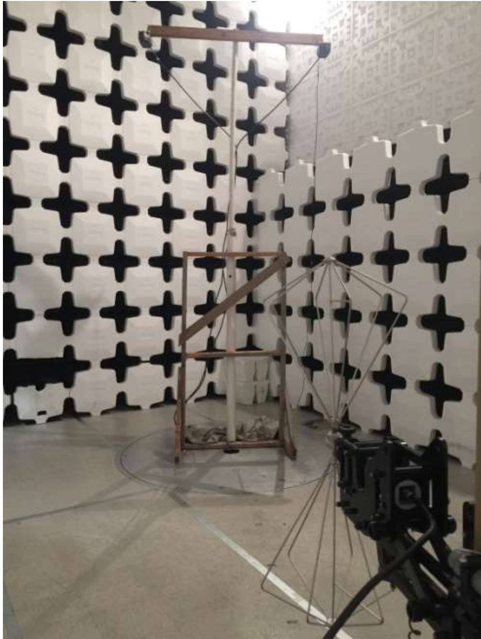
Figure 6. Radiated Emissions, 30-200 MHz, 3.7 Meters
