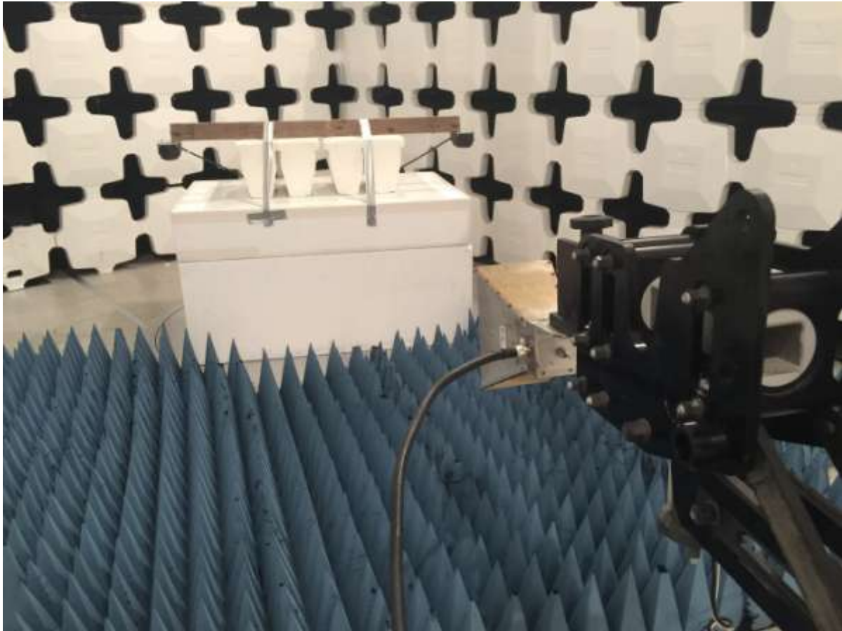
Figure 9. Radiated Emissions, 1 - 6 GHz, 1 Meter
