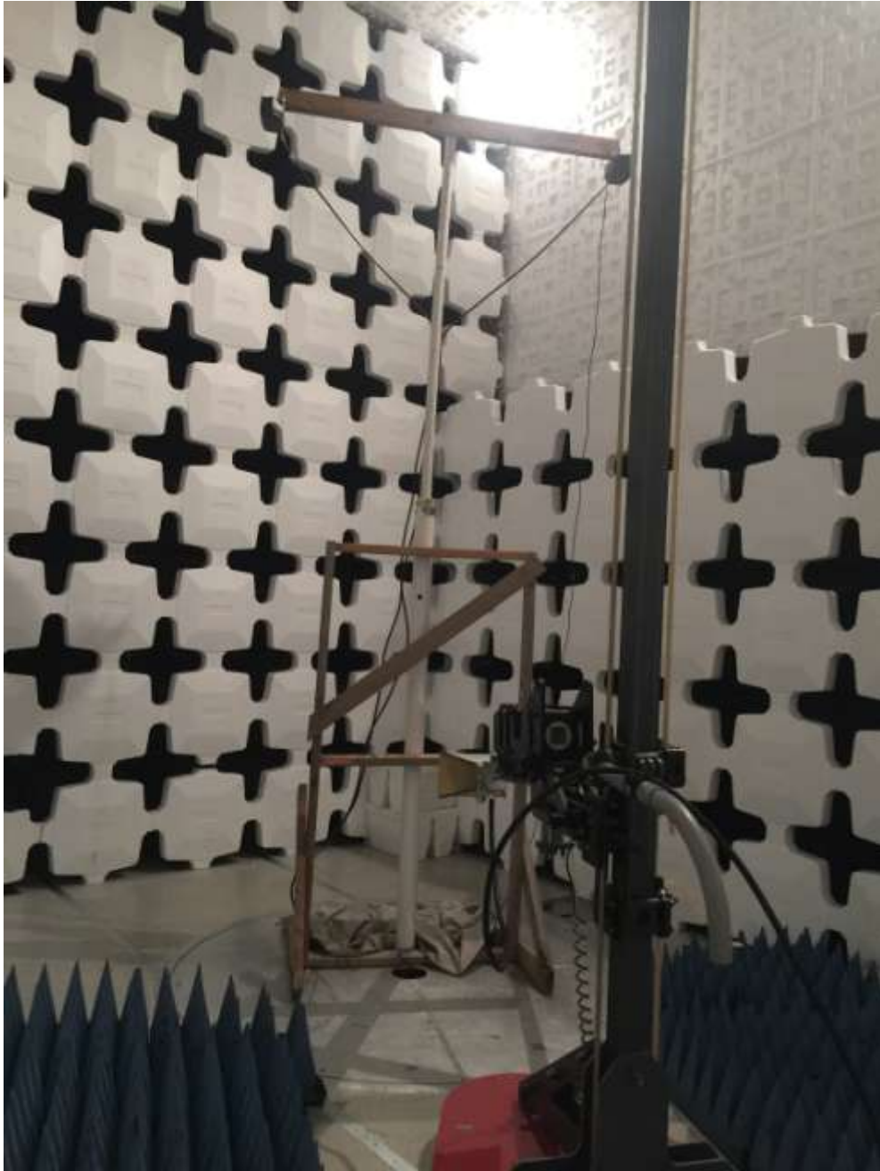
Figure 12. Radiated Emissions, 6 - 18 GHz, 3.7 Meters
