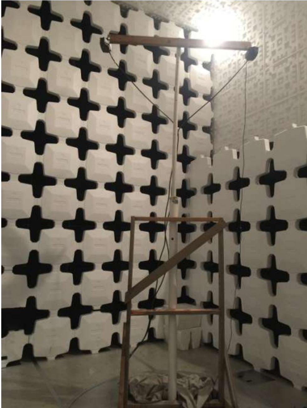
Figure 2. EUT Radiated Emissions Test Setup, 3.7 Meters
