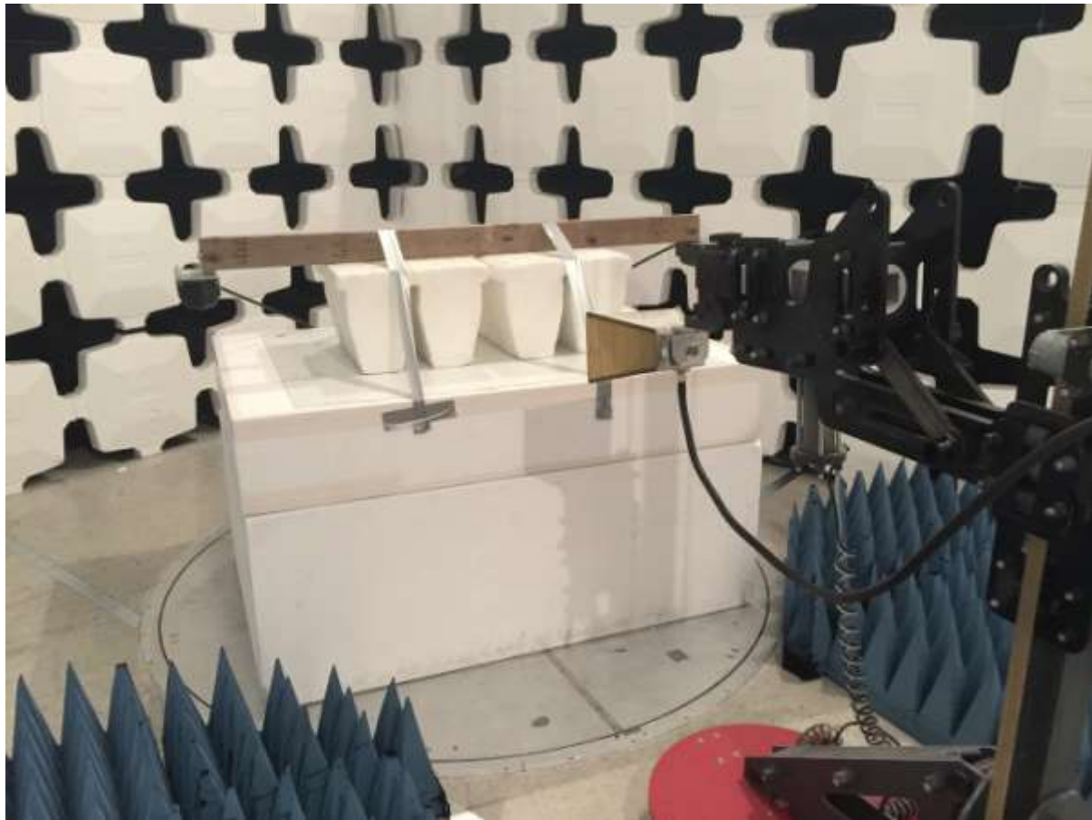
Figure 11. Radiated Emissions, 6 - 18 GHz, 1 Meter
