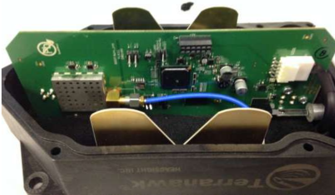
Figure 1. Front Side of PCB in Enclosure
