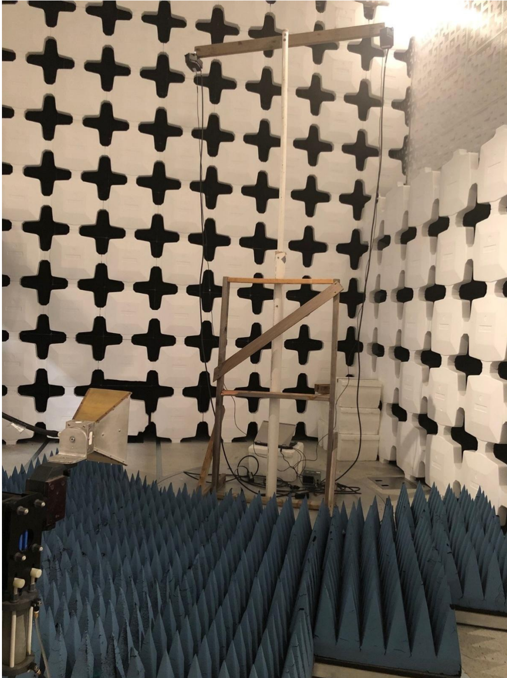
Figure 10. Radiated Emissions, 1 - 6 GHz, 3.7 Meters
