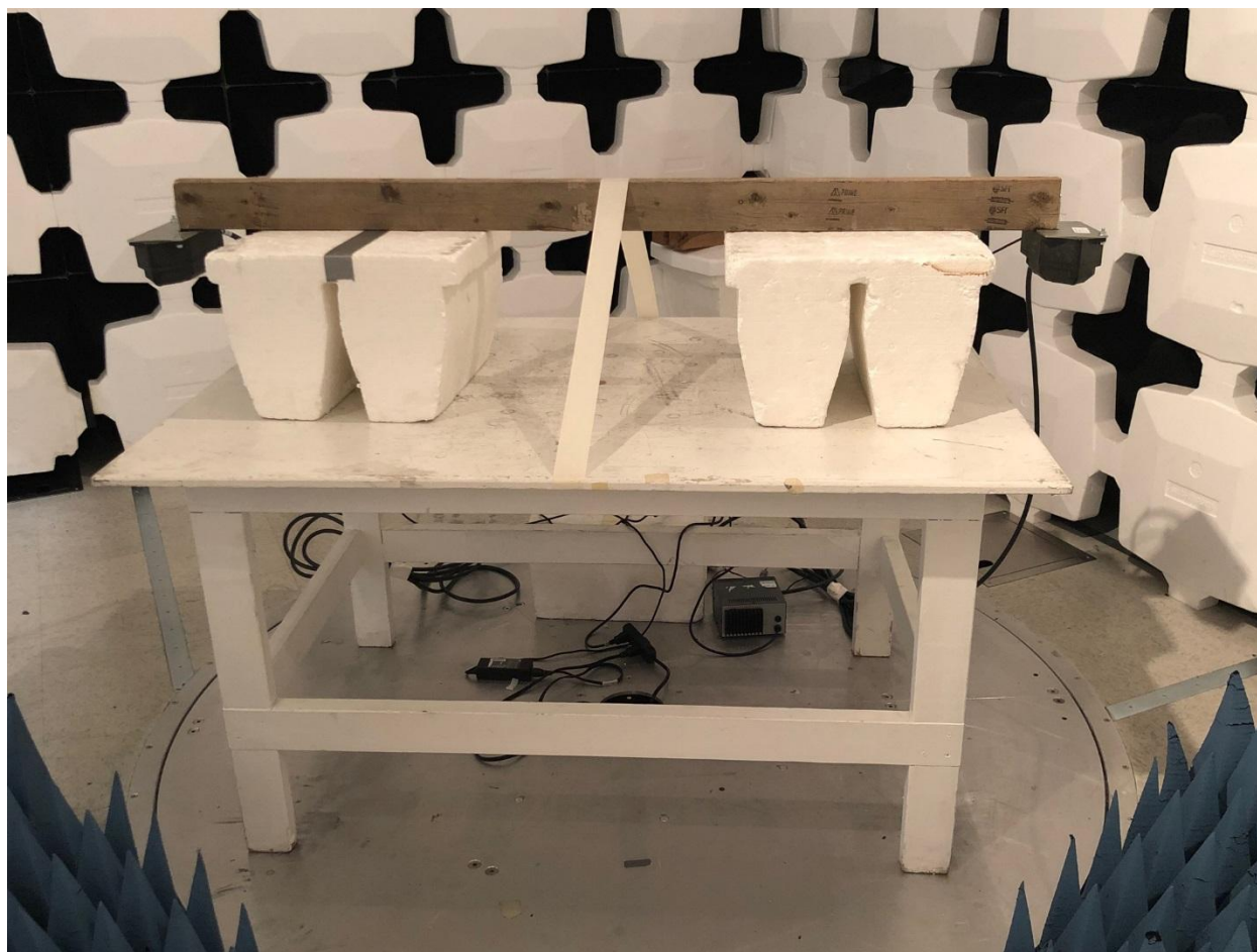
Figure 1. EUT Radiated Emissions Test Setup, 1 Meter
