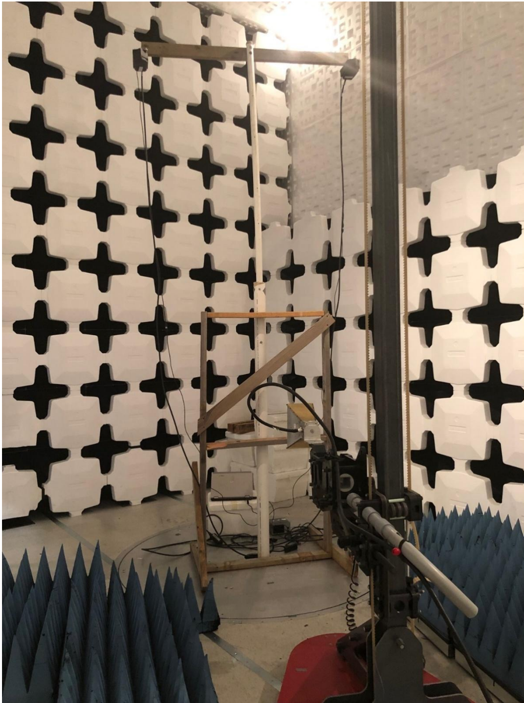
Figure 12. Radiated Emissions, 6 - 18 GHz, 3.7 Meters
