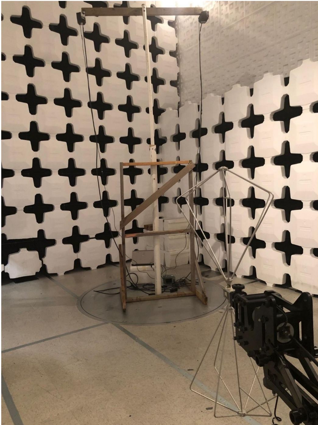
Figure 6. Radiated Emissions, 30-200 MHz, 3.7 Meters
