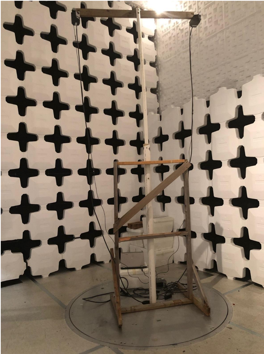
Figure 2.EUT Radiated Emissions Test Setup, 3.7 Meters
