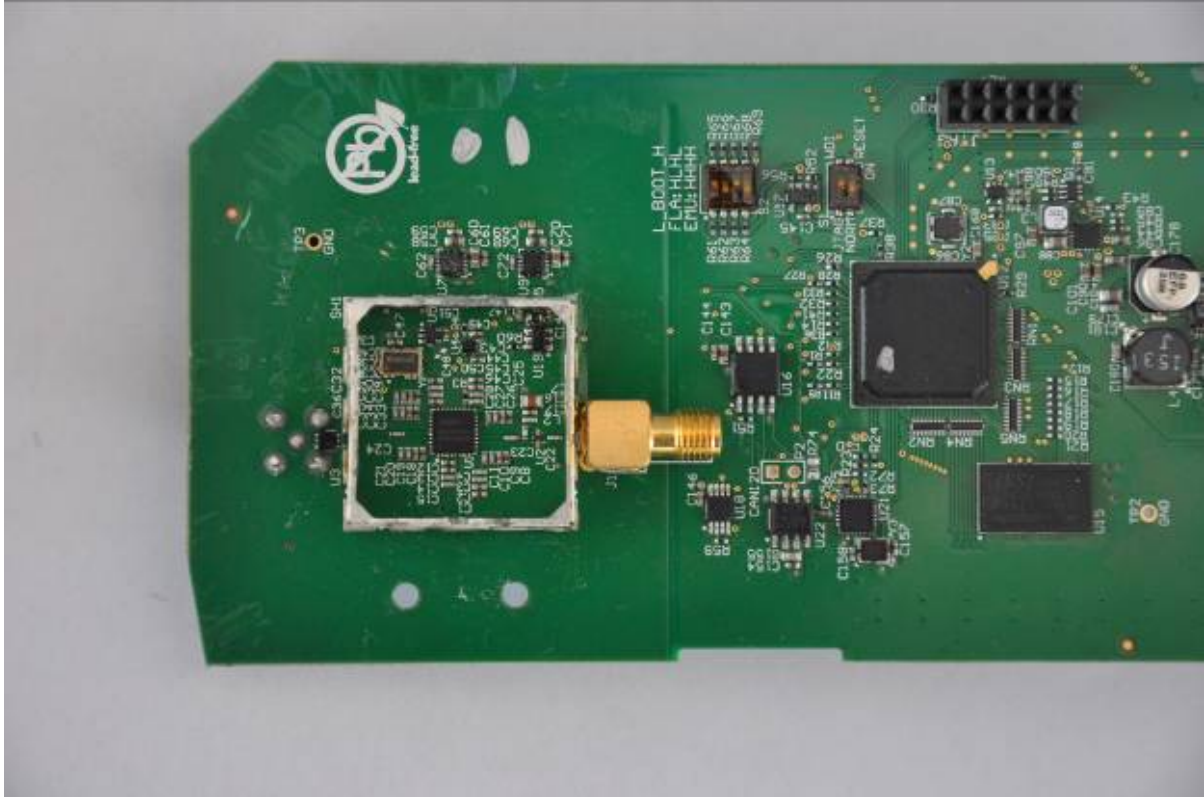
Figure 8. RF Module with Shield Removed
