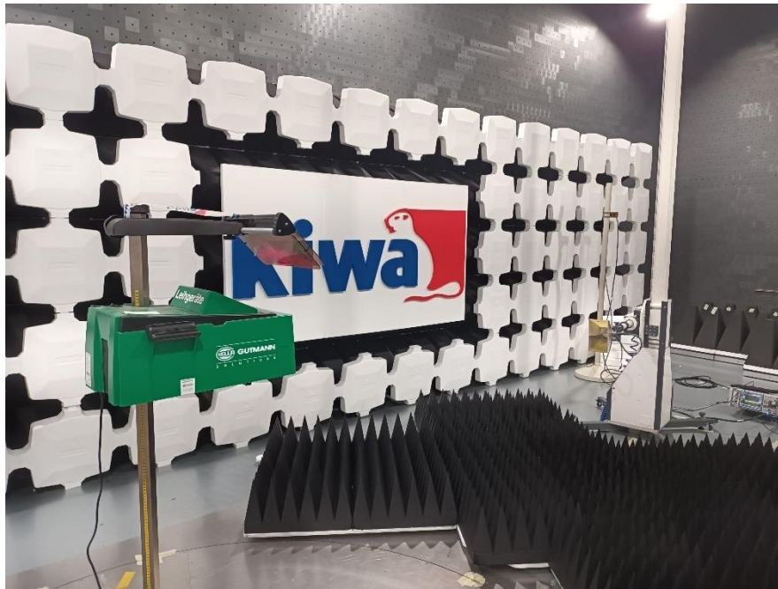
Photo 3 Photograph test setup radiated emissions 1-12.5 GHz, report section 3.1
