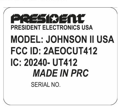
FCC ID plate(serial number) to be fixed to rear-chasis by two rivets.
