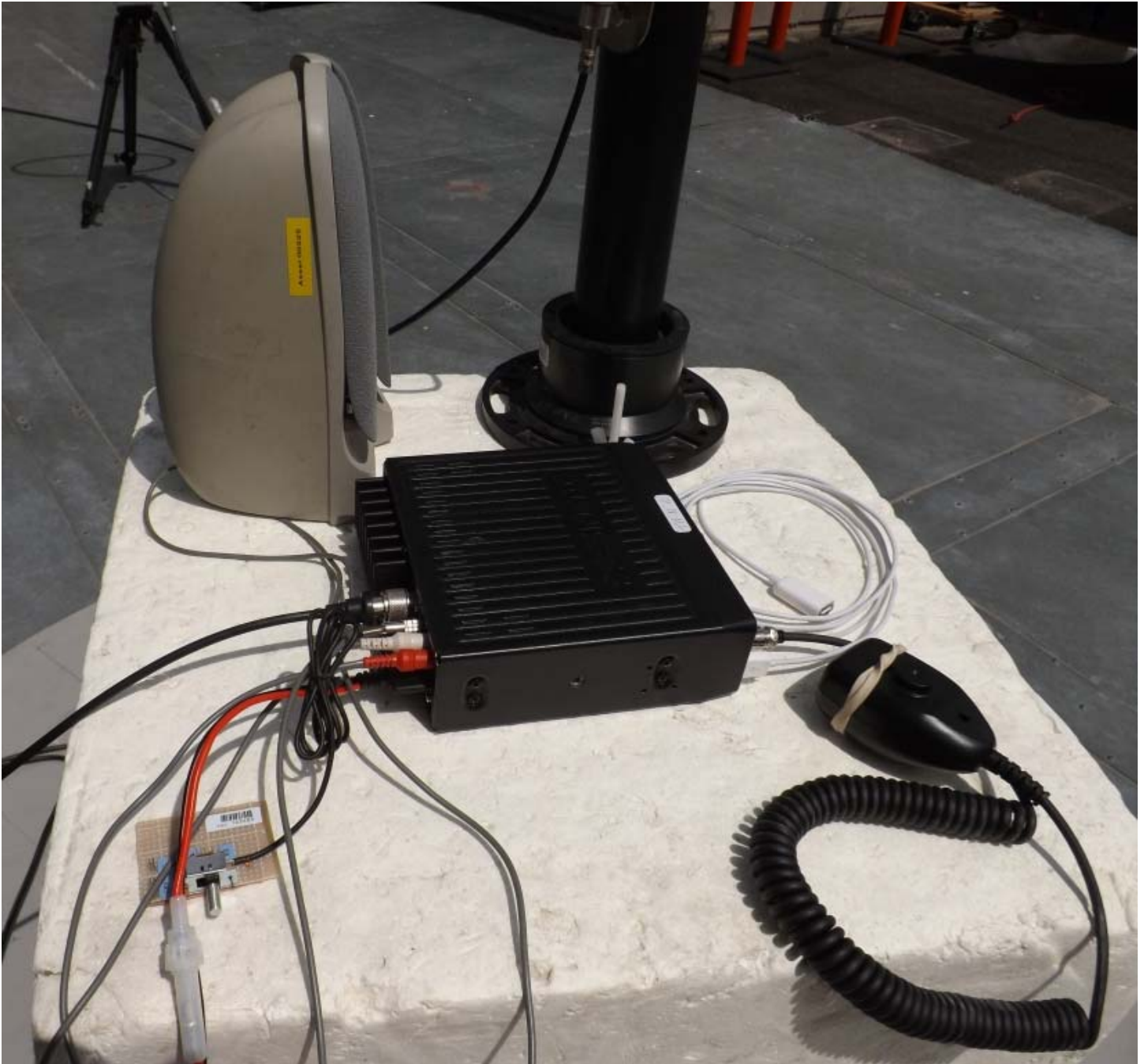
Figure E17.5 – Setup, Radiated Emission with Accessories
