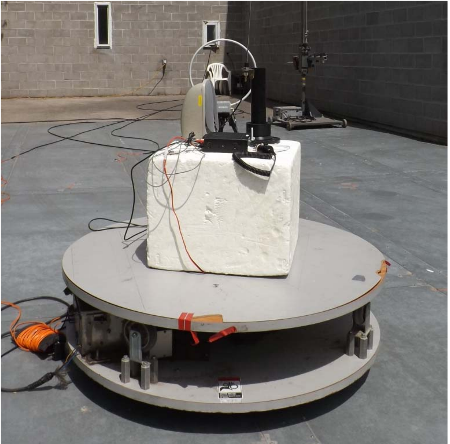
Figure E17.4 – Setup, Radiated Emission < 30MHz, with Accessories
