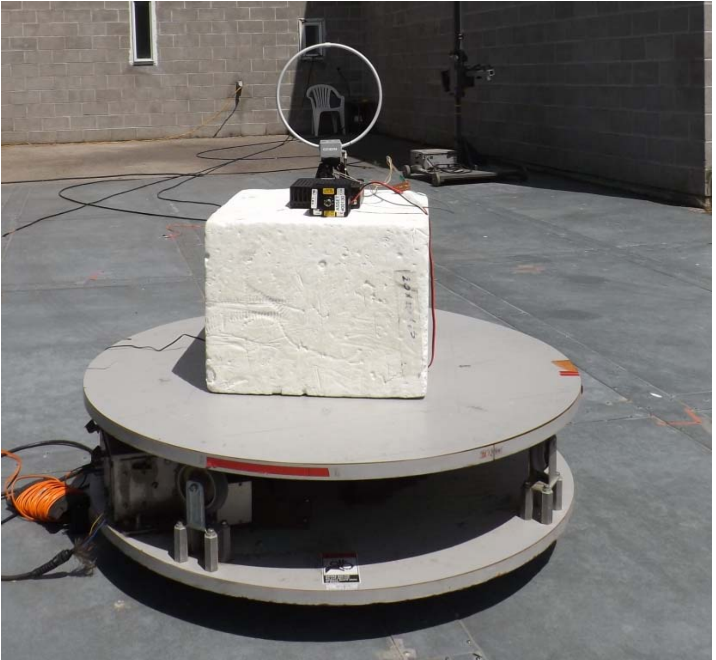
Figure E17.3 – Setup, Radiated Emission < 30MHz, without Accessories
