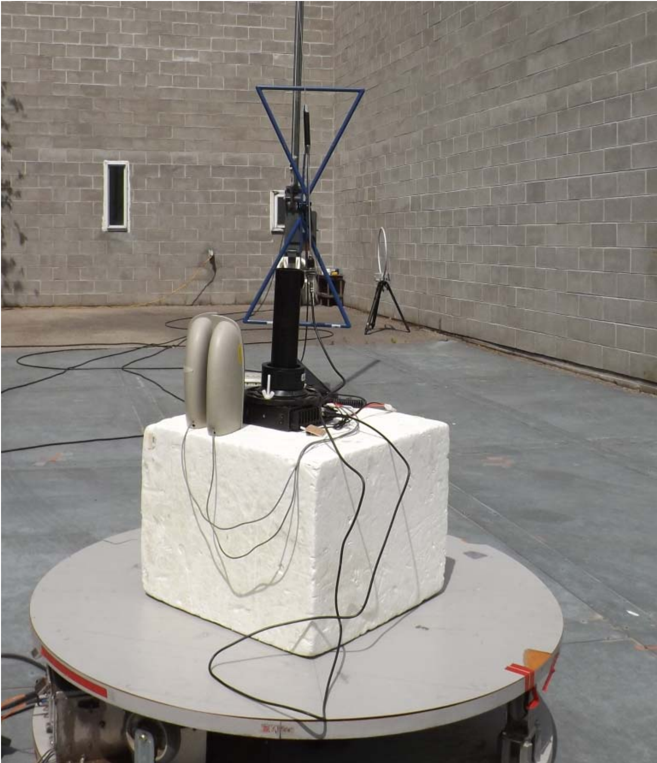
Figure E17.8 – Setup, Radiated Emission, 30 – 1000MHz with Accessories
