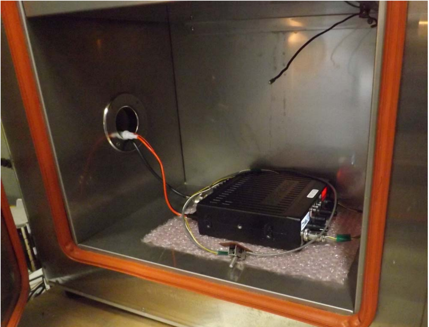
Figure E17.10 – Setup, Frequency Stability
