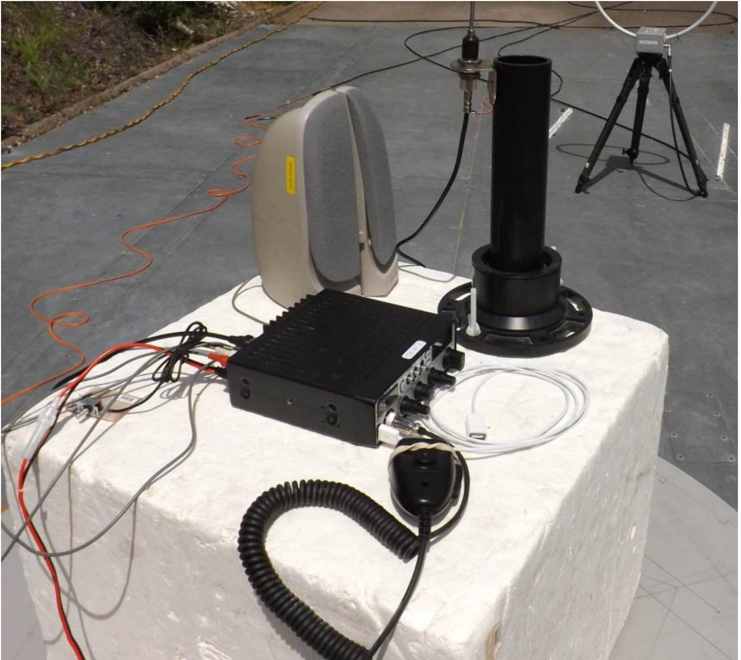
Figure E17.6 – Setup, Radiated Emission with Accessories
