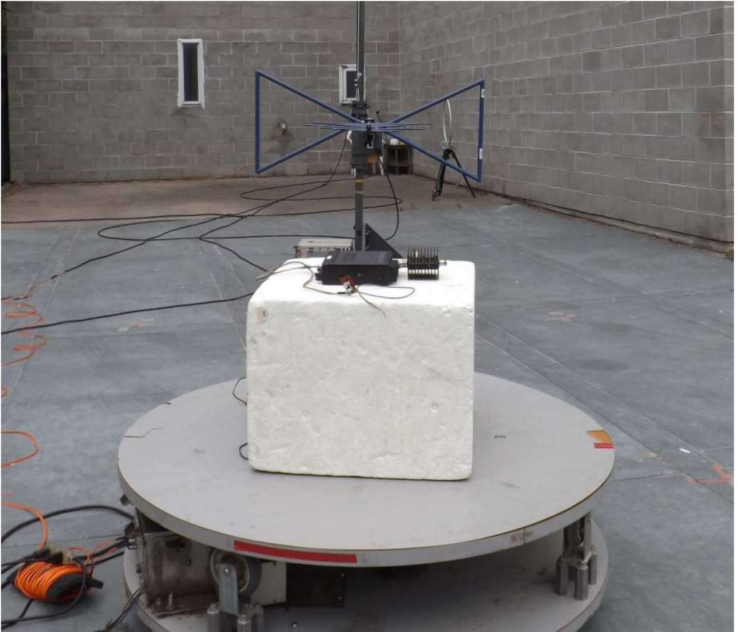
Figure E17.7 – Setup, Radiated Emission, 30 – 1000MHz without Accessories
