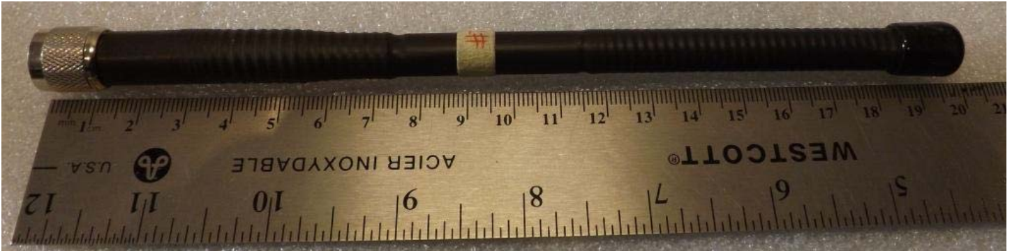
Figure E26.7 – External Photo – Antenna
