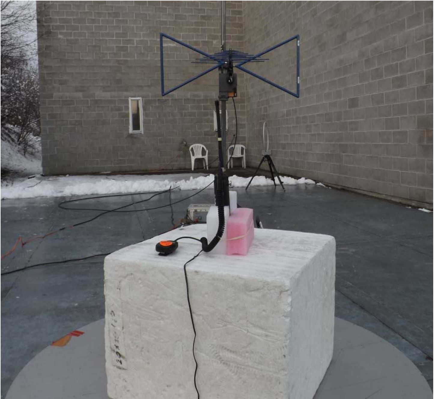
Figure E24.9 – Setup Photo – Radiated Emissions 30 - 1000MHz, Horizontal, With Accessories
