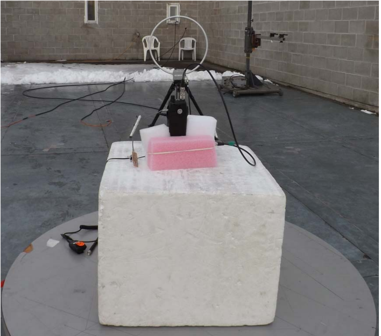
Figure E24.3 – Setup Photo – Radiated Emissions Below 30MHz, Front, Without Accessories
