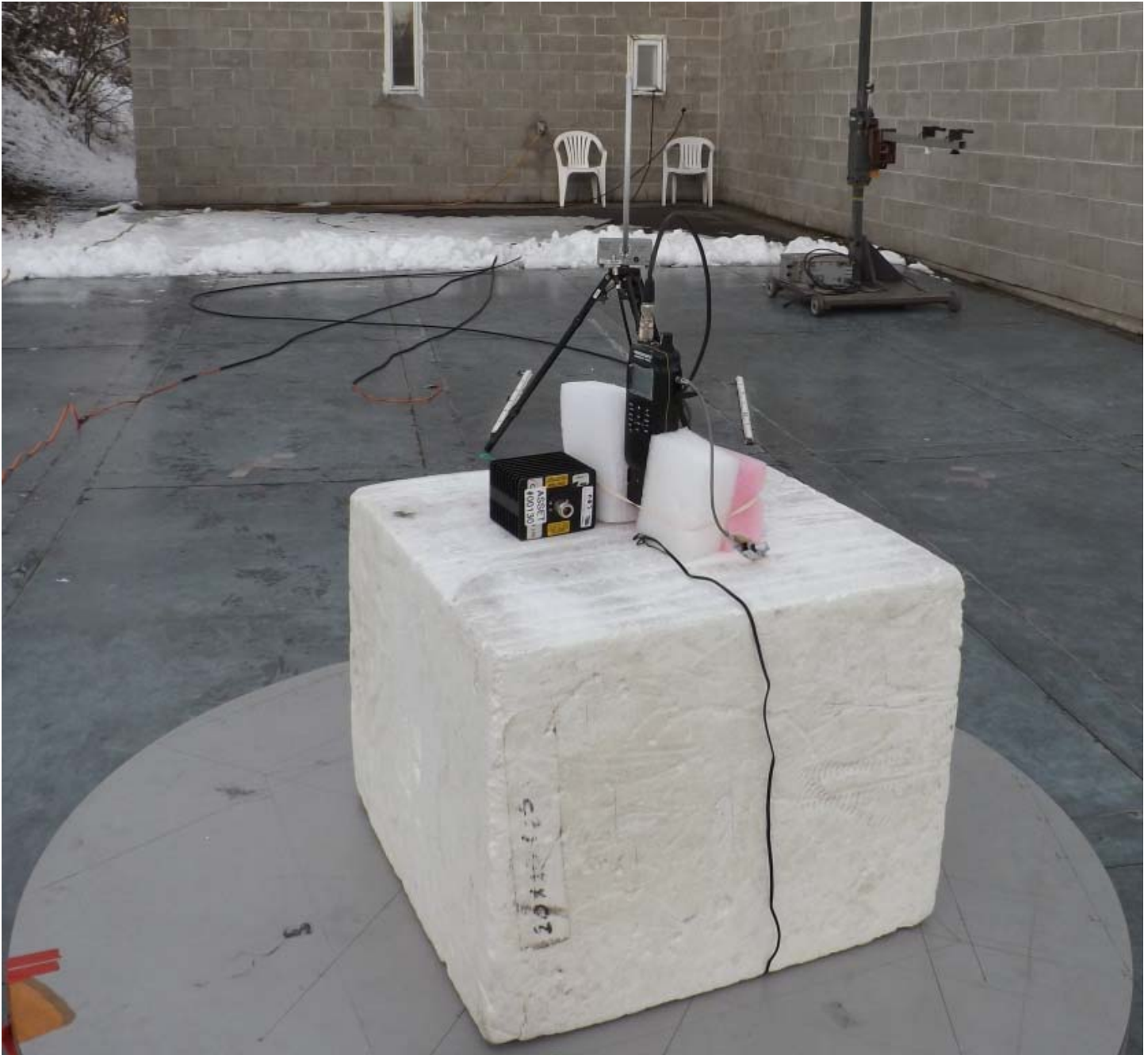
Figure E24.4 – Setup Photo – Radiated Emissions Below 30MHz, Side, Without Accessories
