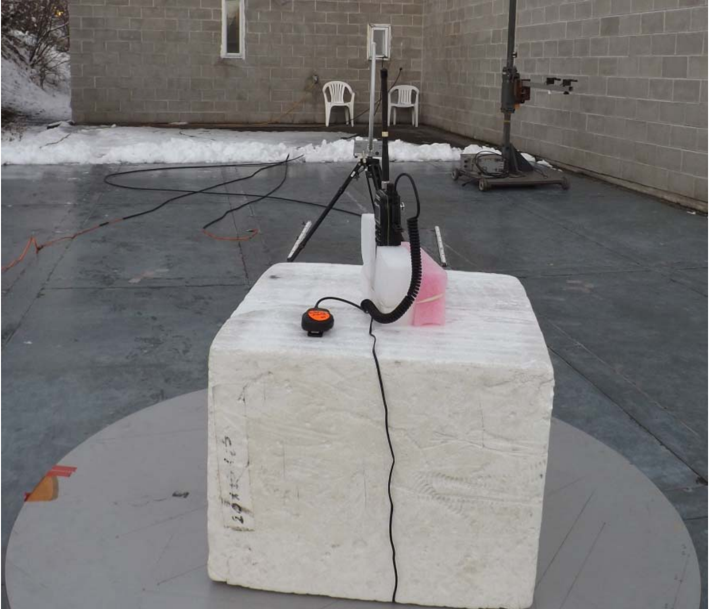
Figure E24.6 – Setup Photo – Radiated Emissions Below 30MHz, Side, With Accessories
