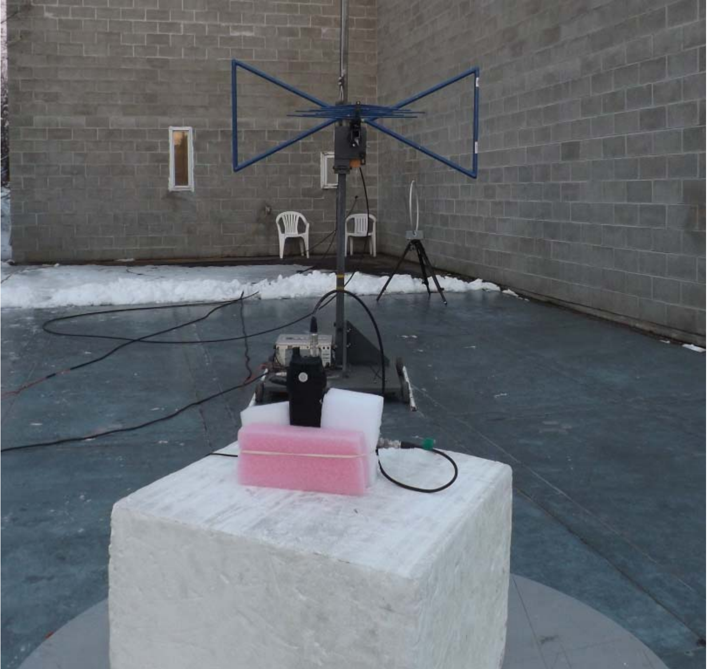
Figure E24.7 – Setup Photo – Radiated Emissions 30 - 1000MHz, Horizontal, Without Accessories
