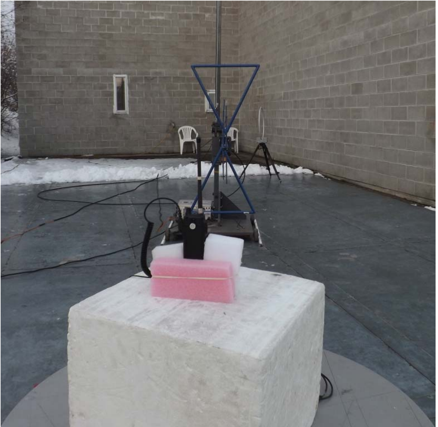
Figure E24.10 – Setup Photo – Radiated Emissions 30 - 1000MHz, Vertical, With Accessories
