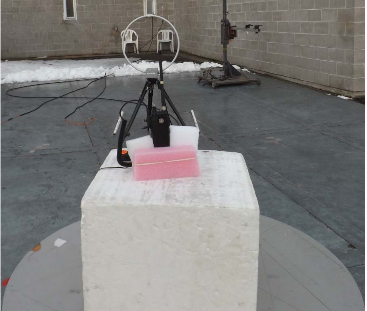
Figure E24.5 – Setup Photo – Radiated Emissions Below 30MHz, Front, With Accessories
