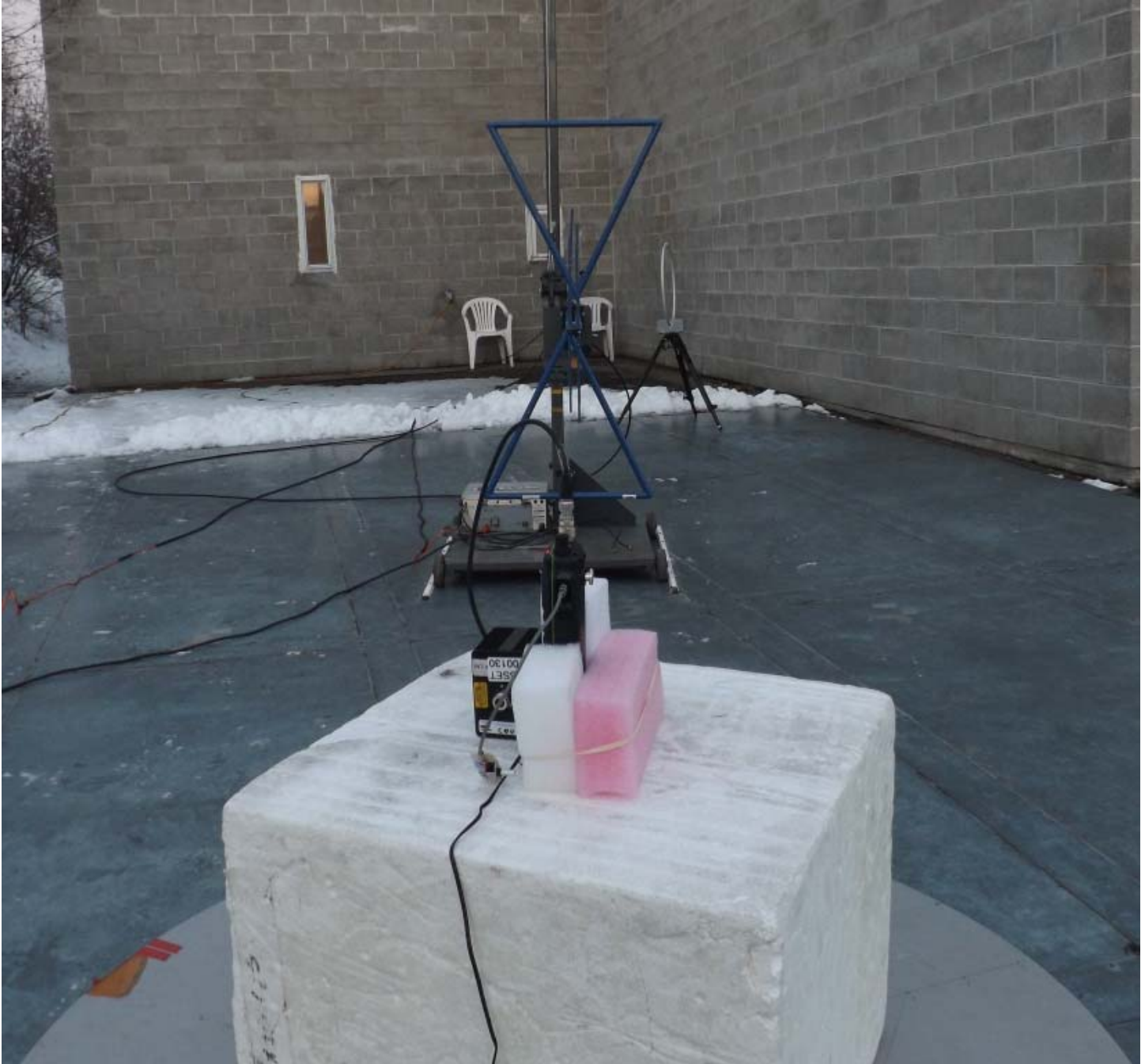
Figure E24.8 – Setup Photo – Radiated Emissions 30 - 1000MHz, Vertical, Without Accessories
