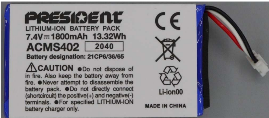
Figure E23.10 – Internal Photo – Battery
