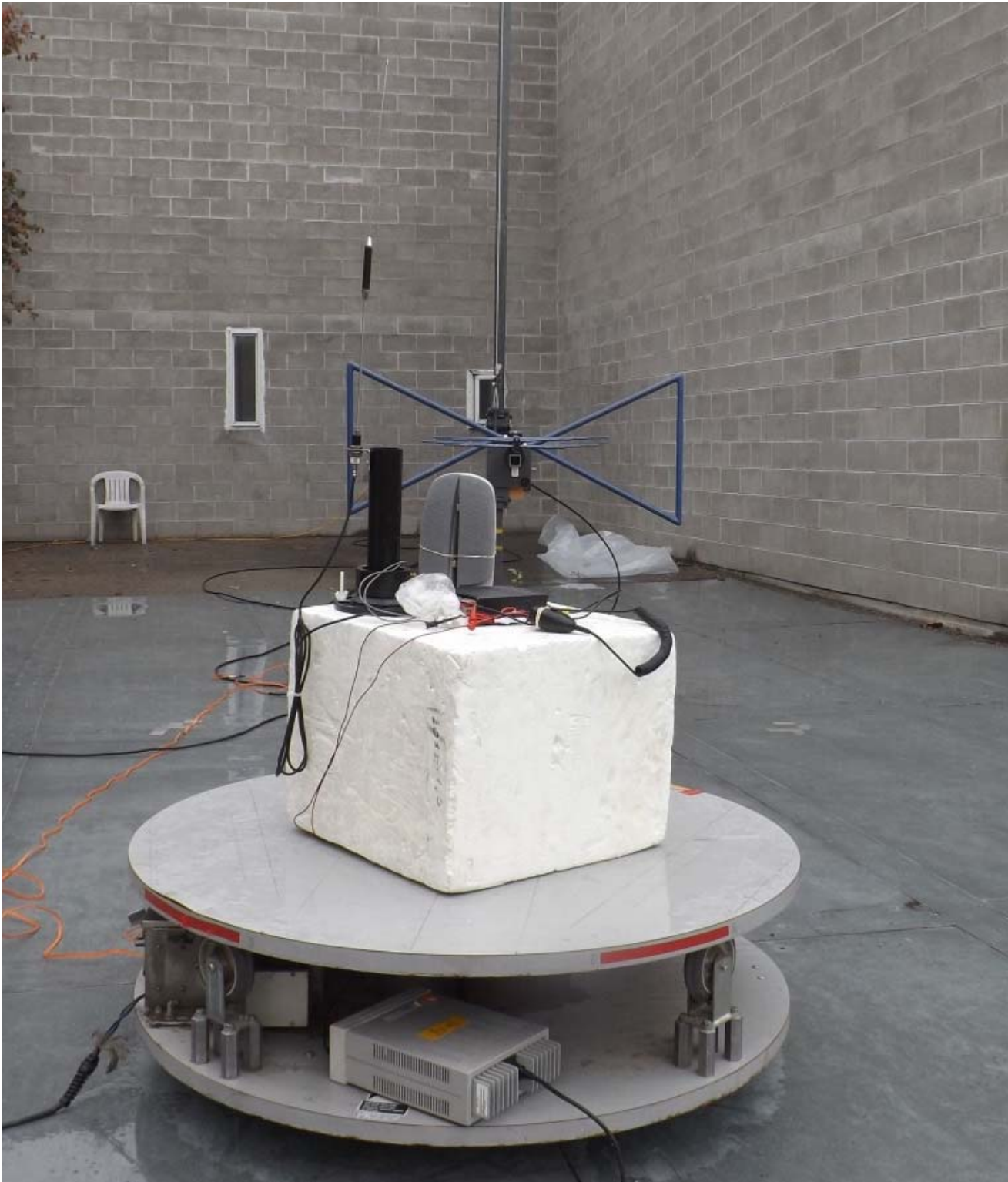
Figure E21.7 – Setup Photo – Radiated Measurements – 30 - 1000MHz Horizontal, with DUT Accessories
