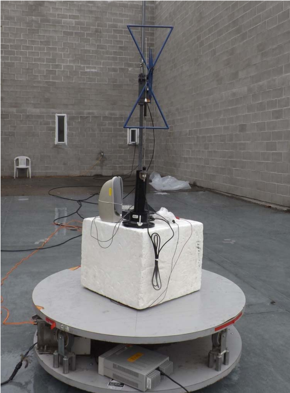
Figure E21.9 – Setup Photo – Radiated Measurements – 30 - 1000MHz Vertical, with DUT Accessories
