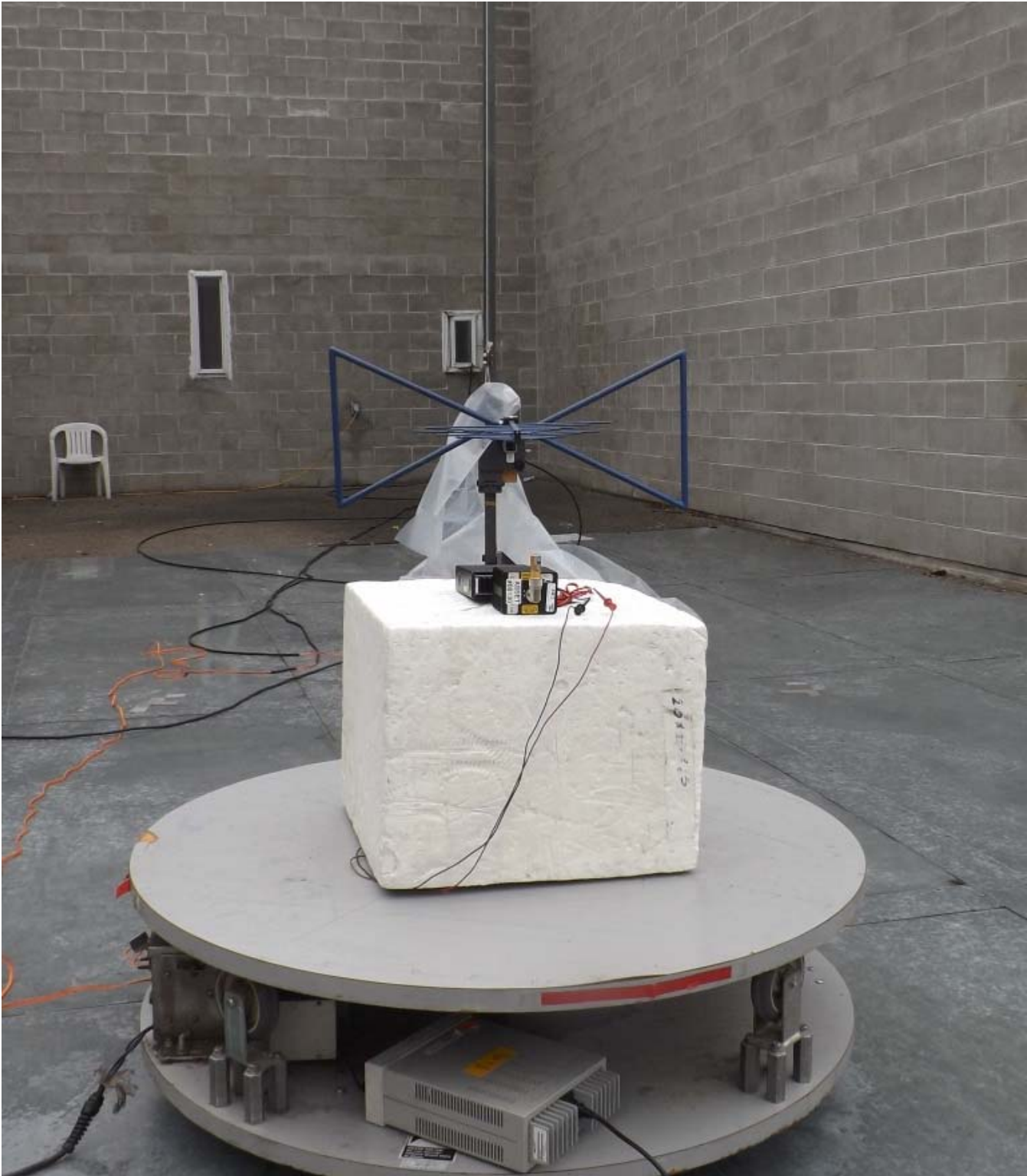
Figure E21.6 – Setup Photo – Radiated Measurements – 30 - 1000MHz Horizontal, without DUT Accessories
