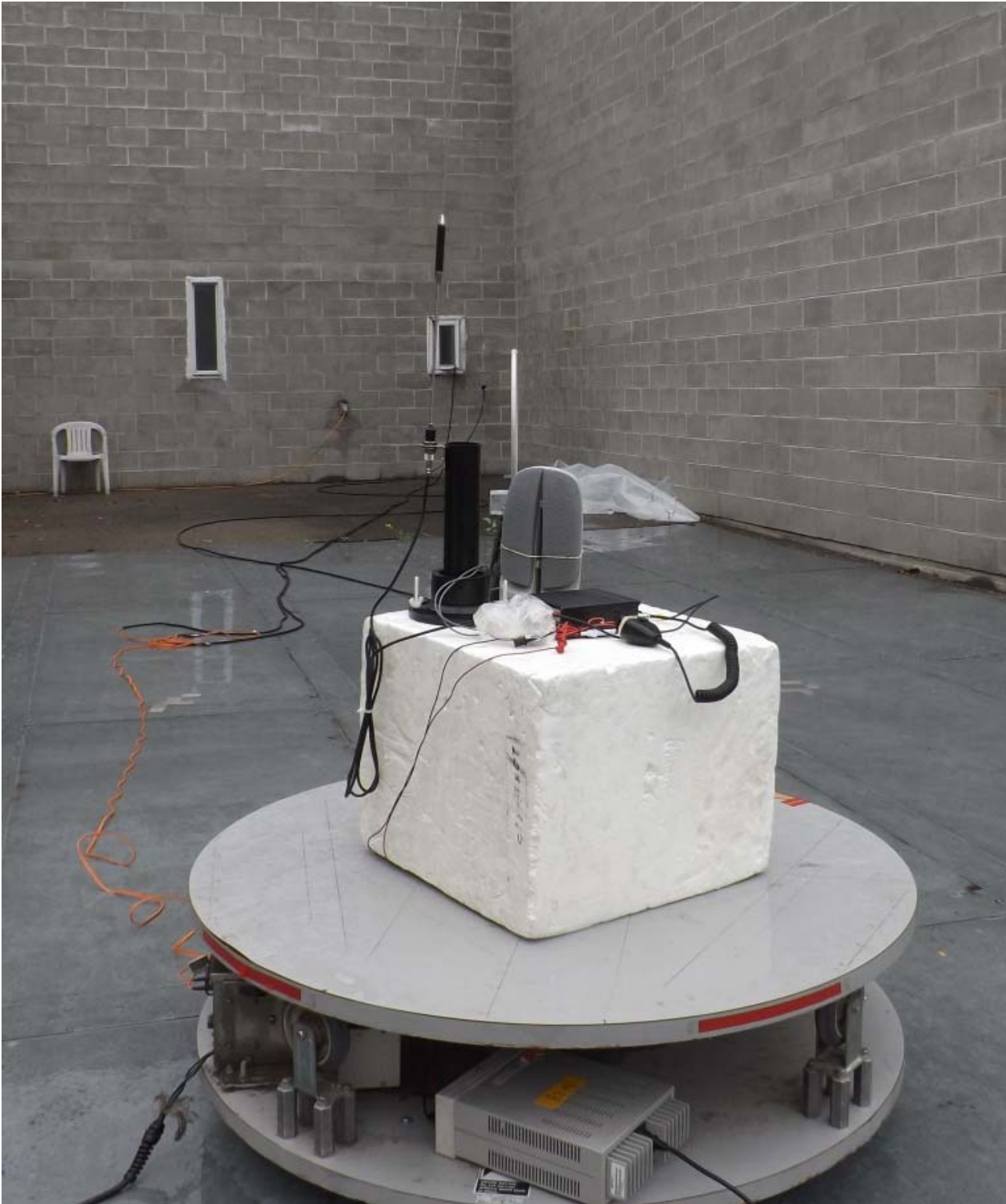
Figure E21.5 – Setup Photo – Radiated Measurements - 9kHz – 30MHz Side, with DUT Accessories
