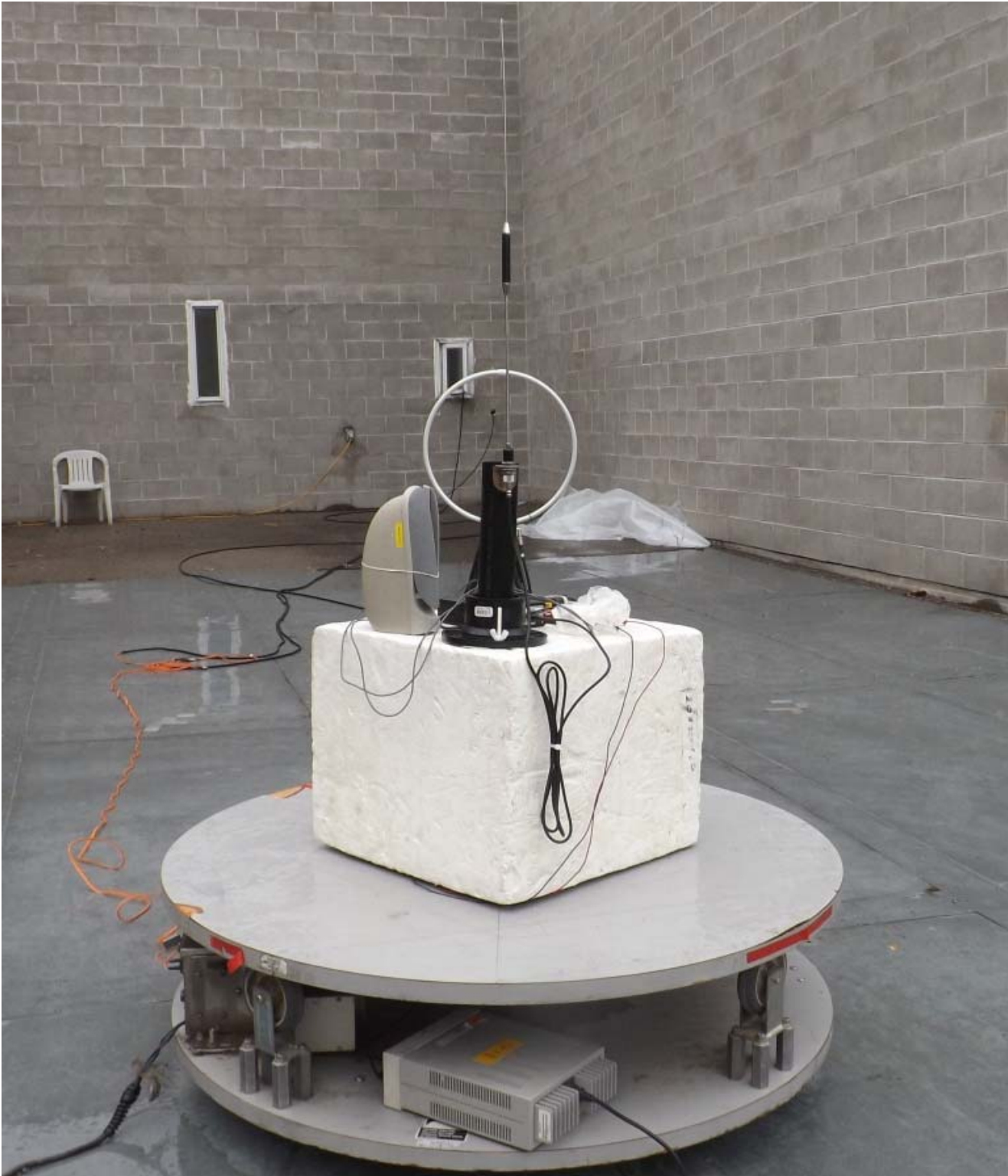
Figure E21.4 – Setup Photo – Radiated Measurements - 9kHz – 30MHz Front, with DUT Accessories
