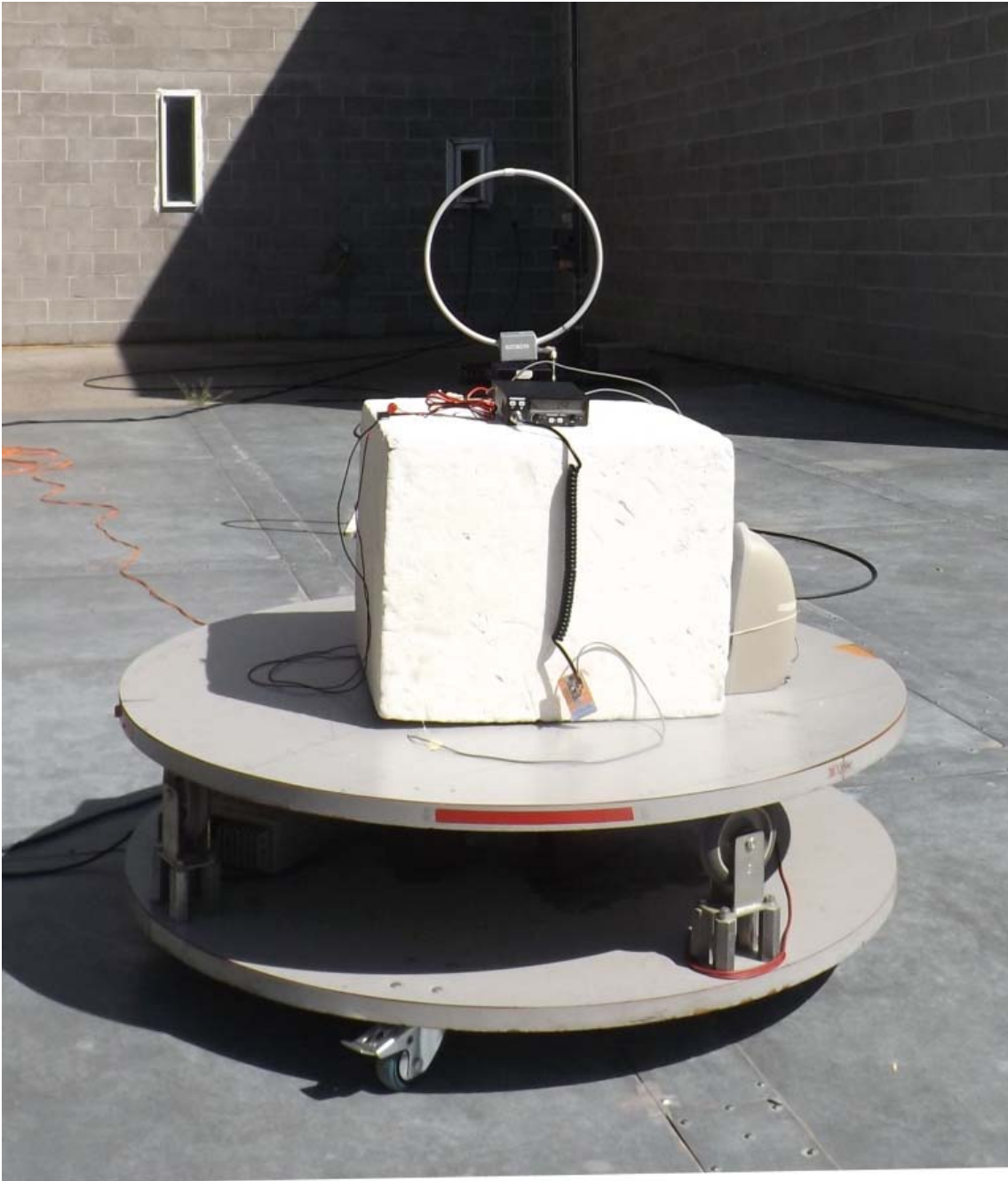
Figure E21.8 – Setup Photo – Radiated Measurements, 9kHz – 30MHz, Front, with Accessories
