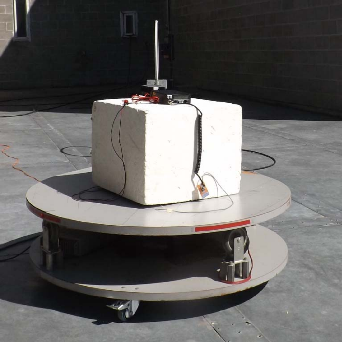
Figure E21.7 – Setup Photo – Radiated Measurements, 9kHz – 30MHz, Side, without Accessories
