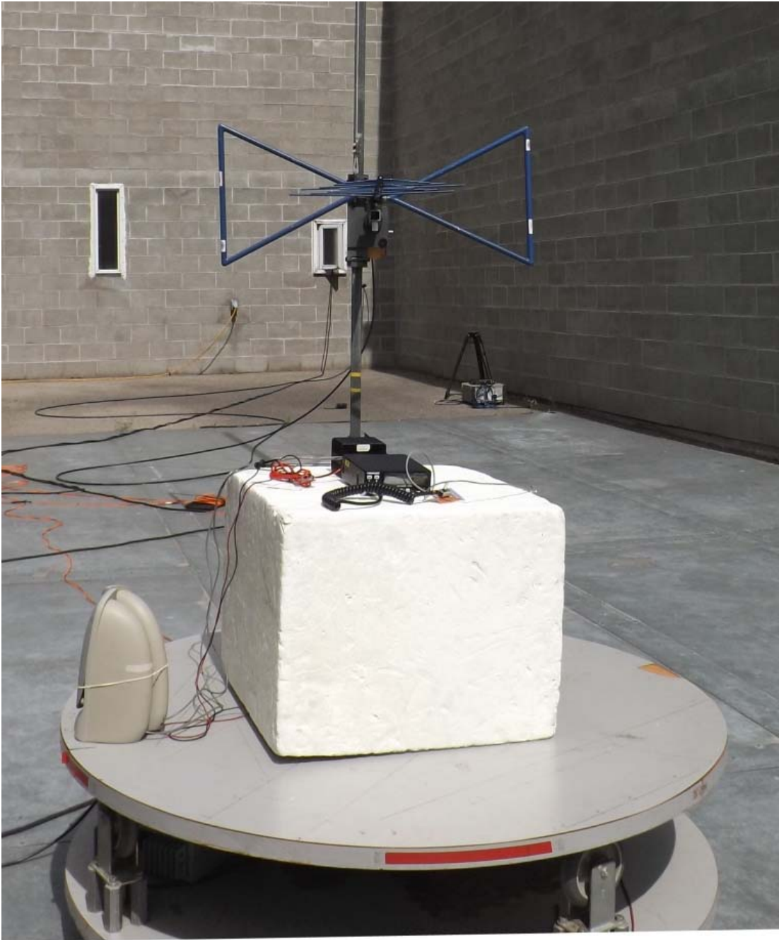
Figure E21.9 – Setup Photo – Radiated Measurements, 30-1000MHz, Horizontal, with Accessories
