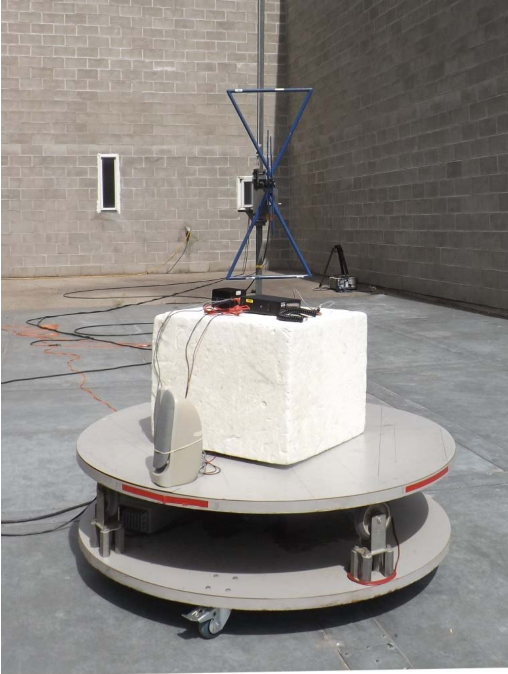
Figure E21.10 – Setup Photo – Radiated Measurements, 30-1000MHz, Vertical, with Accessories
