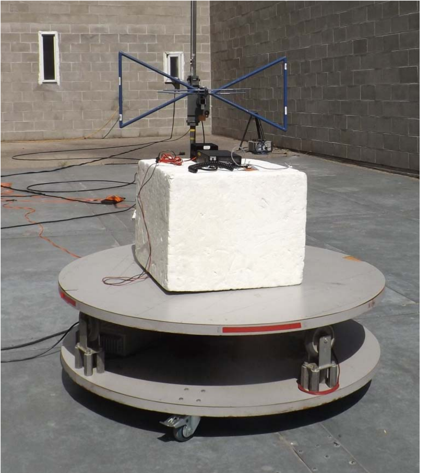
Figure E21.11 – Setup Photo – Radiated Measurements, 30-1000MHz, Horizontal, without Accessories
