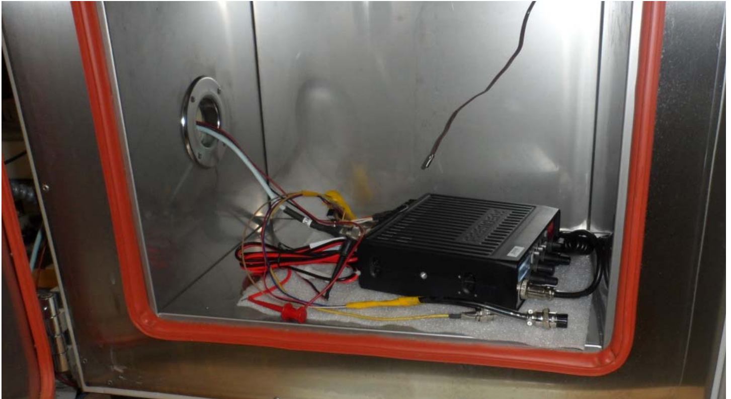
Figure E20.3 – Setup Photo – Frequency Stability Measurements
