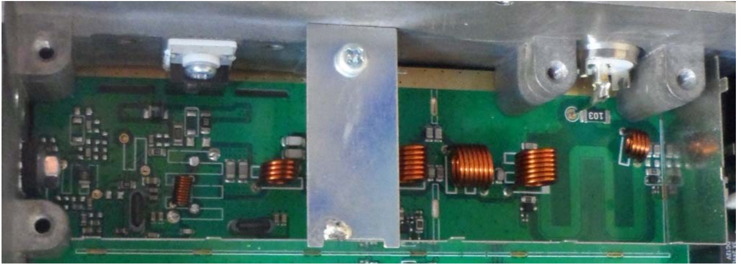
Figure E19.4 – Internal Photo – Main PCB – RF Section
