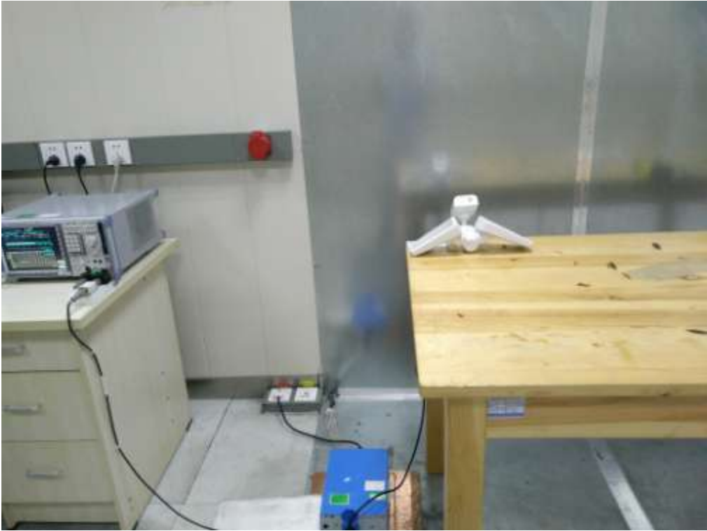
FCC RADIATED EMISSION TEST SETUP BELOW 1GHZ
