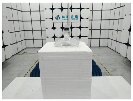
FCC RADIATED EMISSION TEST SETUP ABOVE 1GHZ
