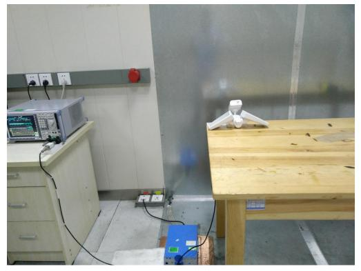
FCC RADIATED EMISSION TEST SETUP BELOW 1GHZ
