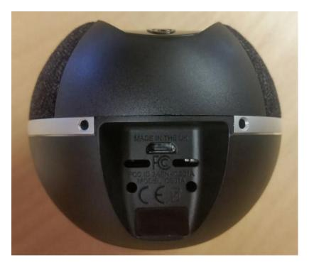
This information moulded into plastic part as part of injection moulding process
