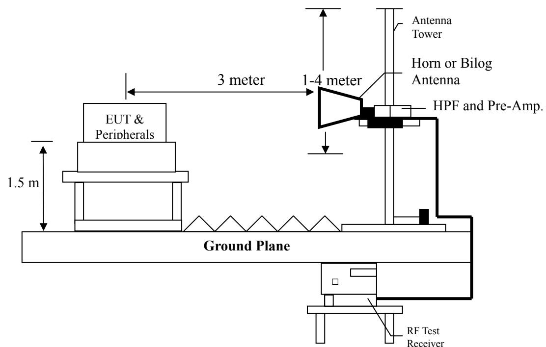
Radiated emissions were invested cover the frequency range from 30MHz to 1000MHz using a receiver RBW of 120kHz record QP reading, and the frequency over 1GHz using a spectrum analyzer RBW of 1MHz and 10Hz VBW record Average reading. (15.209 paragraph), the Peak reading (1 MHz RBW/ 3 MHz VBW) recorded also on the report.
