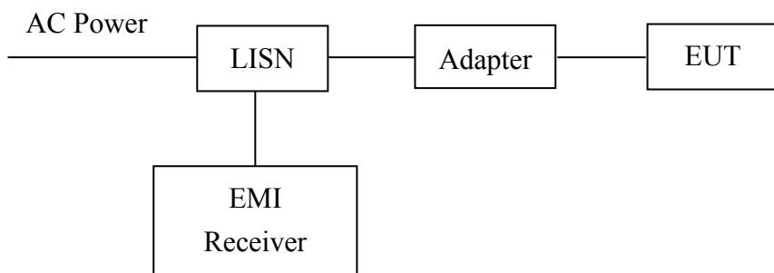
The EUT are connected to the main power through a line impedance stabilization network (LISN). This provides a 50 ohm/50uH coupling impedance for the measuring equipment. The peripheral devices are also connected to the main power through a LISN that provides a 50ohm/50uH coupling impedance with 50ohm termination.
