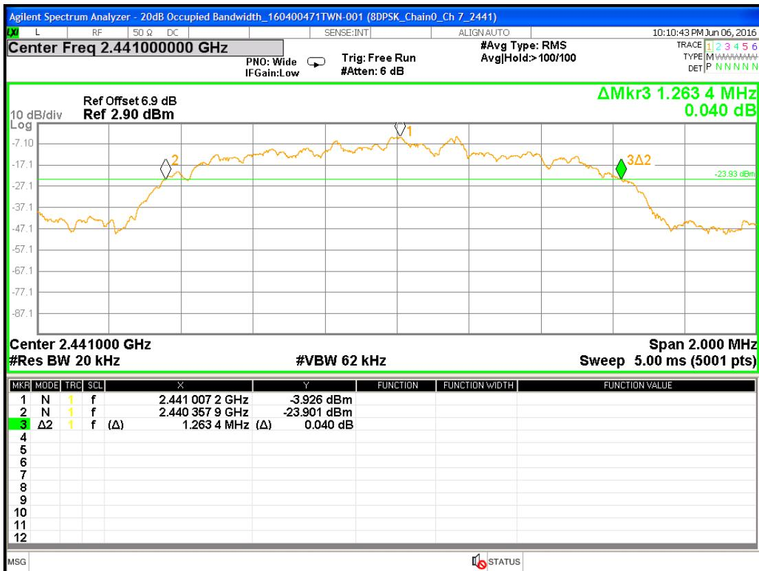
20dB Occupied Bandwidth @ 8DPSK mode Channel 78 2480MHz
