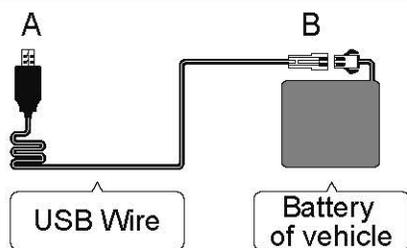
It takes 4 to 5 hours to fully charge the battery at rated voltage. The charge time shall not exceed 10 hours.
