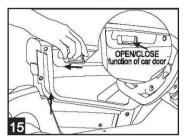
Red (yellow) button inside is for OPEN/CLOSE function of car door. When pushing the button backward and pulling the button upward to the top, the door will open (Please see Picture 15).
