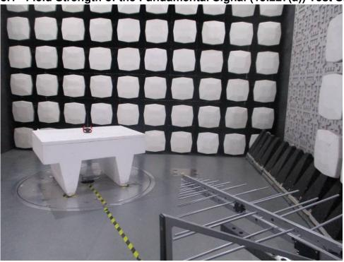
8.2 Radiated Emissions(9kHz-30MHz) Test Setup
