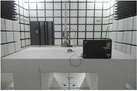
Radiated Emission Setup Photos (30MHz~1GHz)
