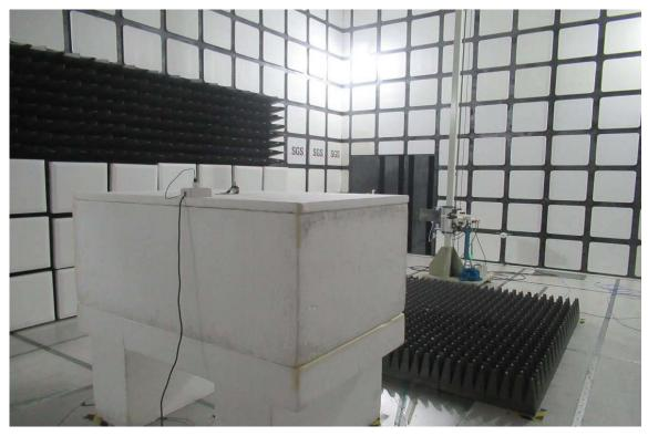
Radiated Emission Set up Photos (Front View)
