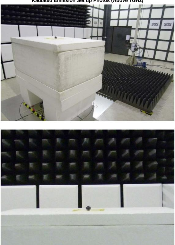
Radiated Emission Set up Photos (Above 1GHz)
