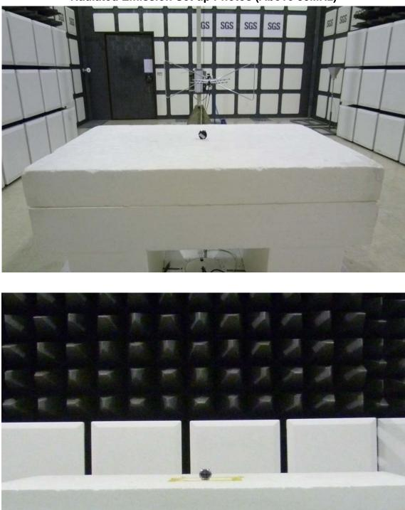
Radiated Emission Set up Photos (Above 30MHz)
