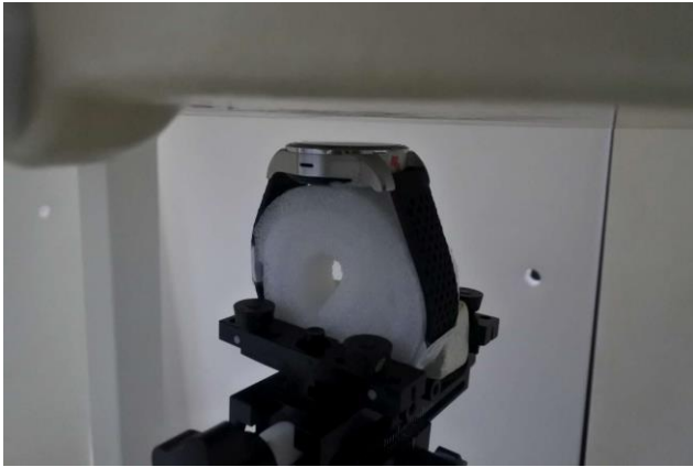
Next to the mouth, Test Separation 10 mm
