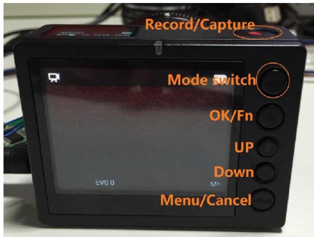
Press the “Mode switch” button will switch the camera mode under the sequence:
