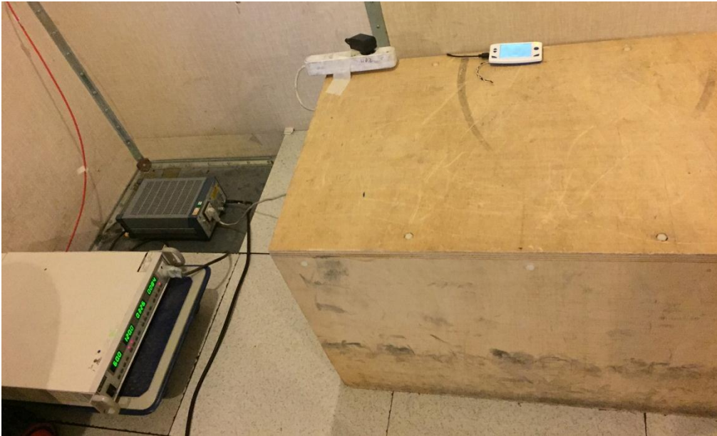
Test set up of conducted emission on power supply
