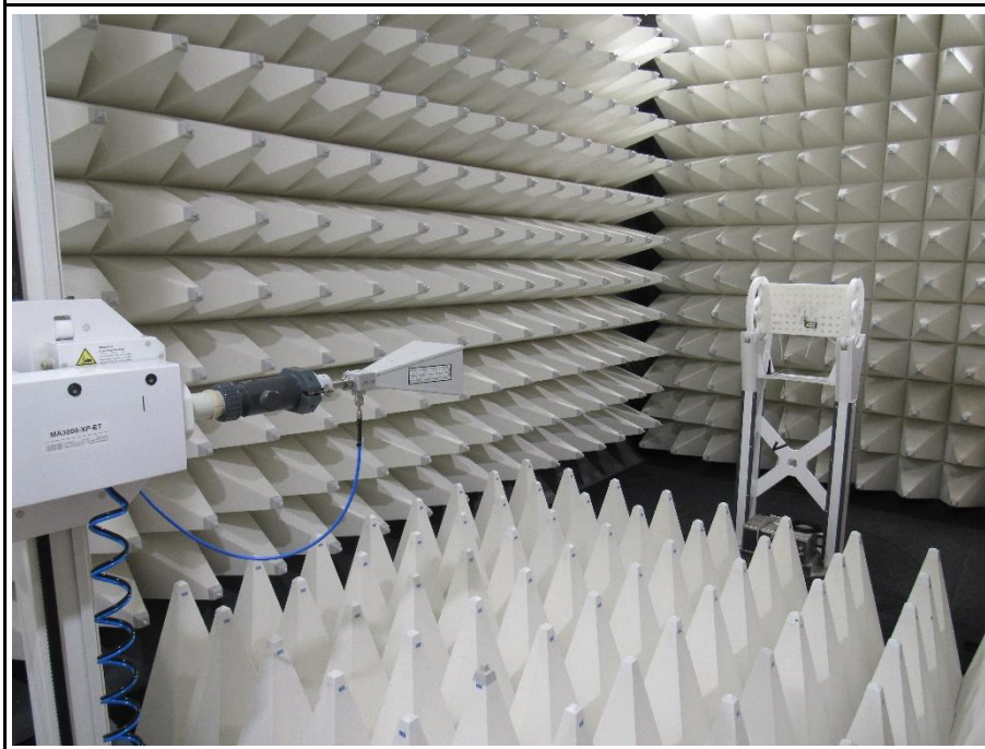
Setup for measurements above 1 GHz
