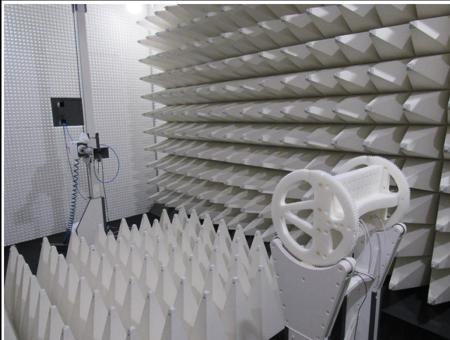
Setup for measurements above 1 GHz
