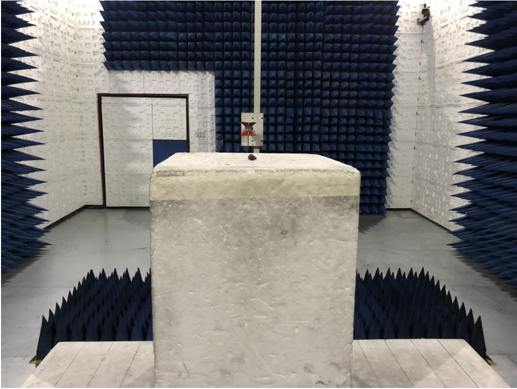
RADIATED EMISSION TEST SETUP ABOVE 1GHZ
