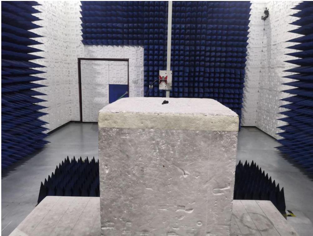
RADIATED EMISSION TEST SETUP ABOVE 1GHz
