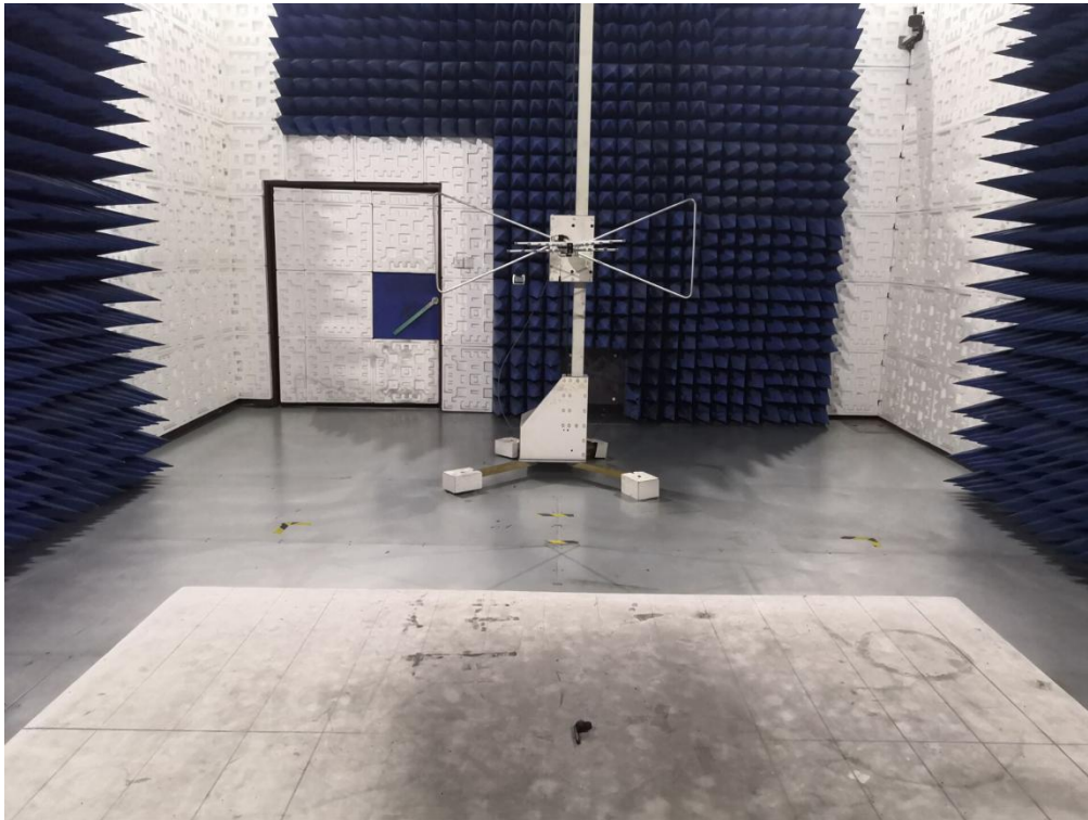
RADIATED EMISSION TEST SETUP ABOVE 1GHz
